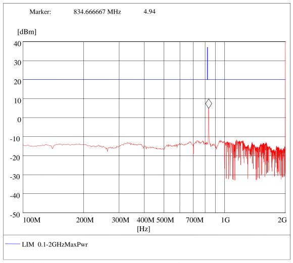
Unmodulated Emissions Masks: Test Results Output Power Setup #2 of 2
