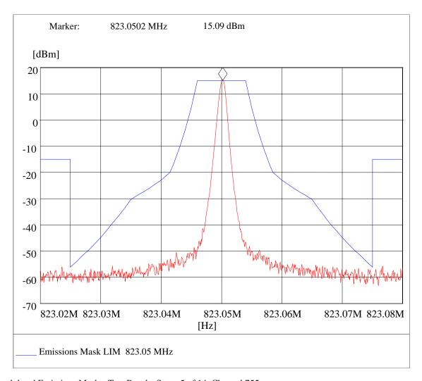
Unmodulated Emissions Masks: Test Results <u>Setup 5 of 14, Channel 755</u>
