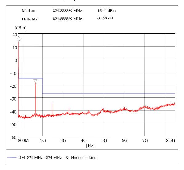
Unmodulated Spurious Emissions: Test Results Output Power & Harmonics from Forward Power
