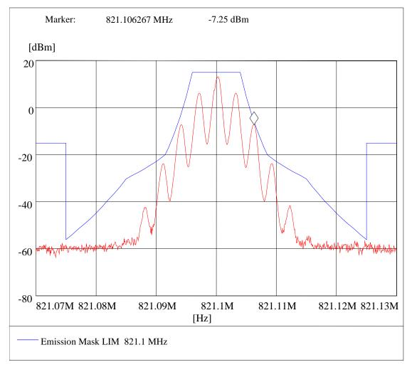
Modulated Emissions Masks: Test Results Setup 2 of 14, Channel 607
