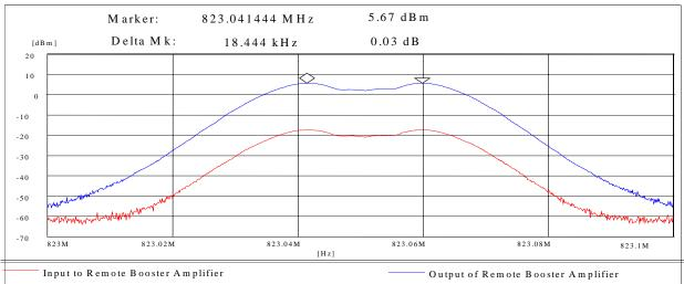
FM Modulated Emissions: Input and Output Power Comparison
