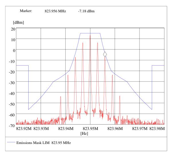
Modulated Emissions Masks: EUT Output Test Results, <u>Setup 12 of 14, Channel 825</u>
