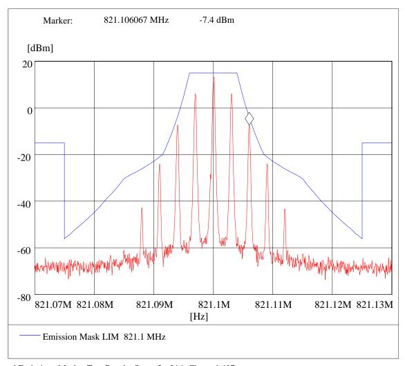
Modulated Emissions Masks: Test Results Setup 3 of 14, Channel 607
