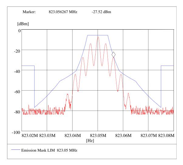
Modulated Emissions Masks: Generator Output Test Results, Setup 9 of 14, Channel 755
