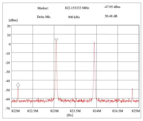
Intermodulation Emissions: Remote Booster Output Power Forward Channel Setup
