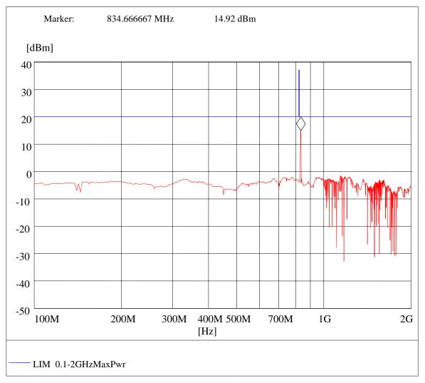
Unmodulated Emissions Masks: Test Results Output Power Setup #1 of 2
