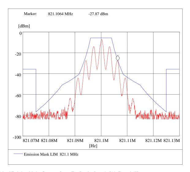
Modulated Emissions Masks: Generator Output Test Results, Setup 4 of 14, Channel 607
