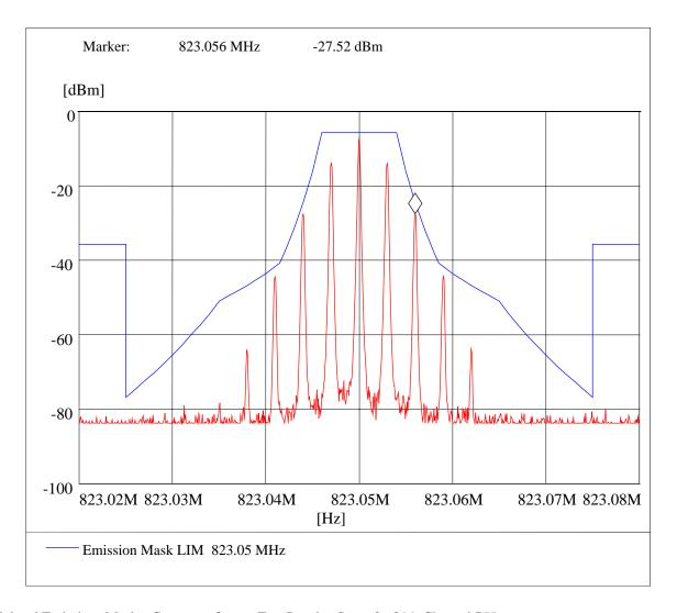
Modulated Emissions Masks: Generator Output Test Results, Setup 8 of 14, Channel 755
