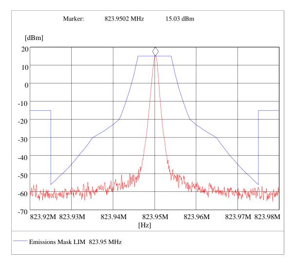
Unmodulated Emissions Masks: Test Results Setup 10 of 14, Channel 825
