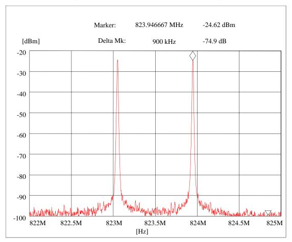
Intermodulation Emissions: Signal Generator Output Reverse Channel Setup
