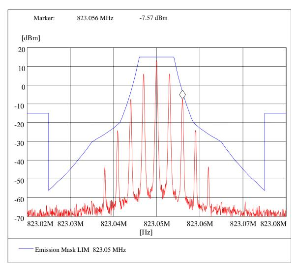
Modulated Emissions Masks: EUT Output Test Result, Setup 7 of 14, Channel 755
