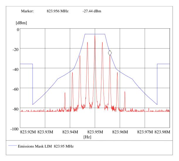
Modulated Emissions Masks: Generator Output Test Results, <u>Setup 13 of 14, Channel 825</u>
