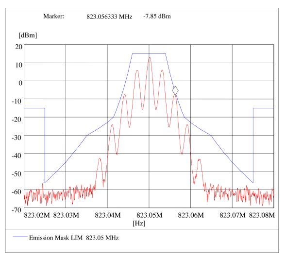
Modulated Emissions Masks: EUT Output Test Results, Setup 6 of 14, Channel 755
