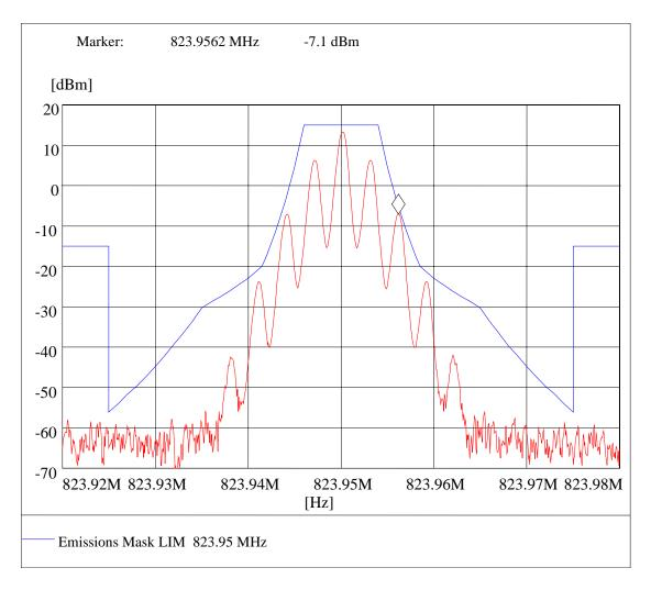
Modulated Emissions Masks: EUT Output Test Results, <u>Setup 11 of 14</u>, <u>Channel 825</u>
