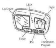
If a gross out of balance condition causes the door to stop while closing, the out of balance condition MUST be corrected before the door can be lowered by the operator. Constant pressure on the Up/Down button will not allow the door to be lowered in this condition. See Troubleshooting Section.
