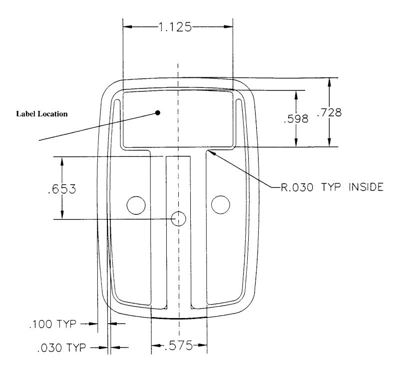
Label Location Drawing. Actual size of label is 1.11"X.58" and will be placed on the back panel of the enclosure.
