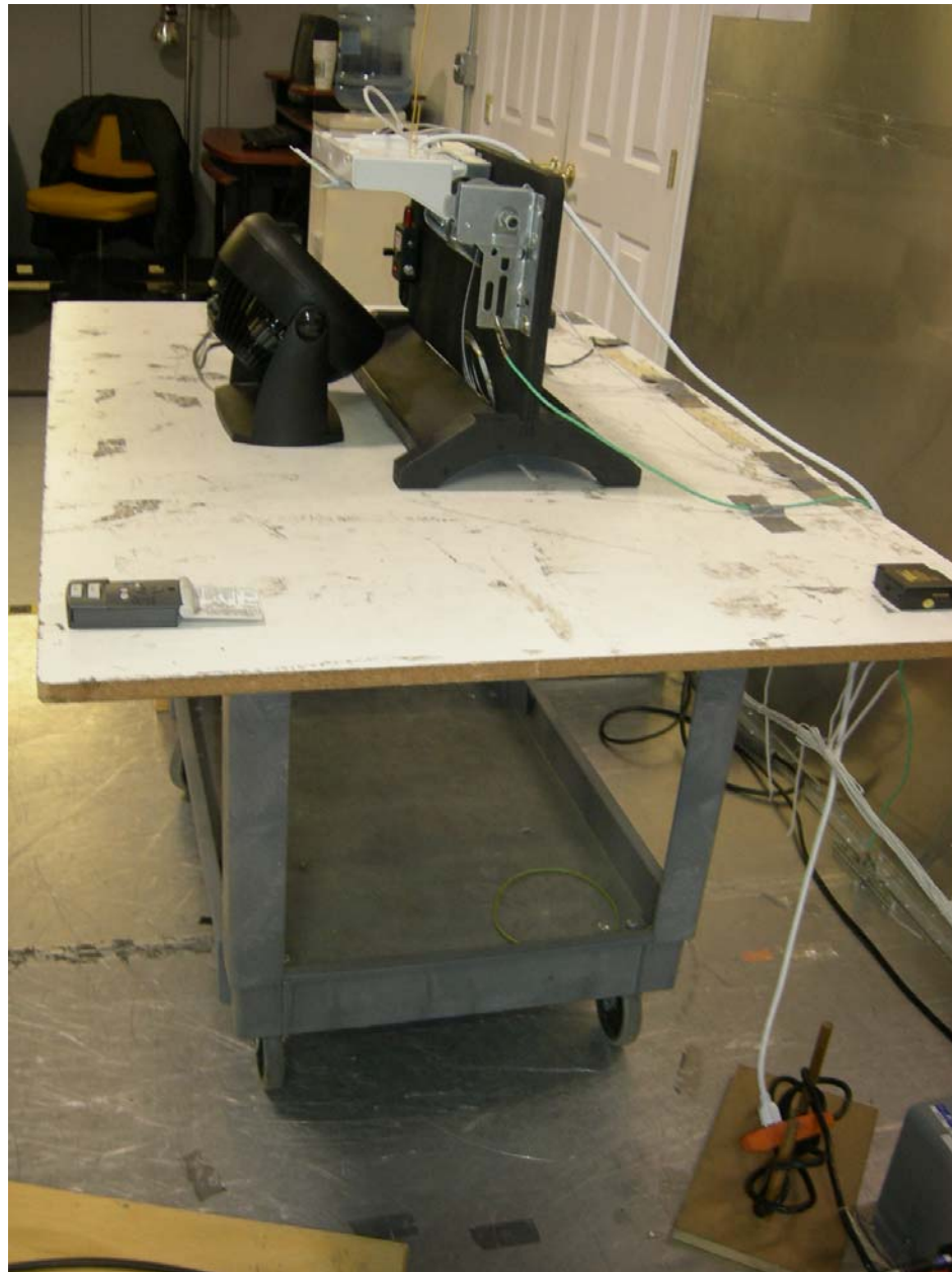
Figure 6: AC Power Line Conducted Emissions
