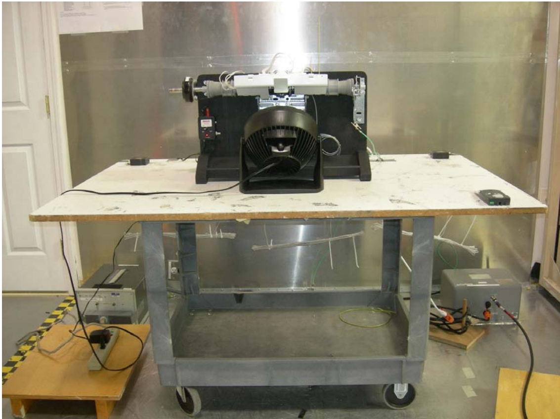
Figure 4: AC Power Line Conducted Emissions
