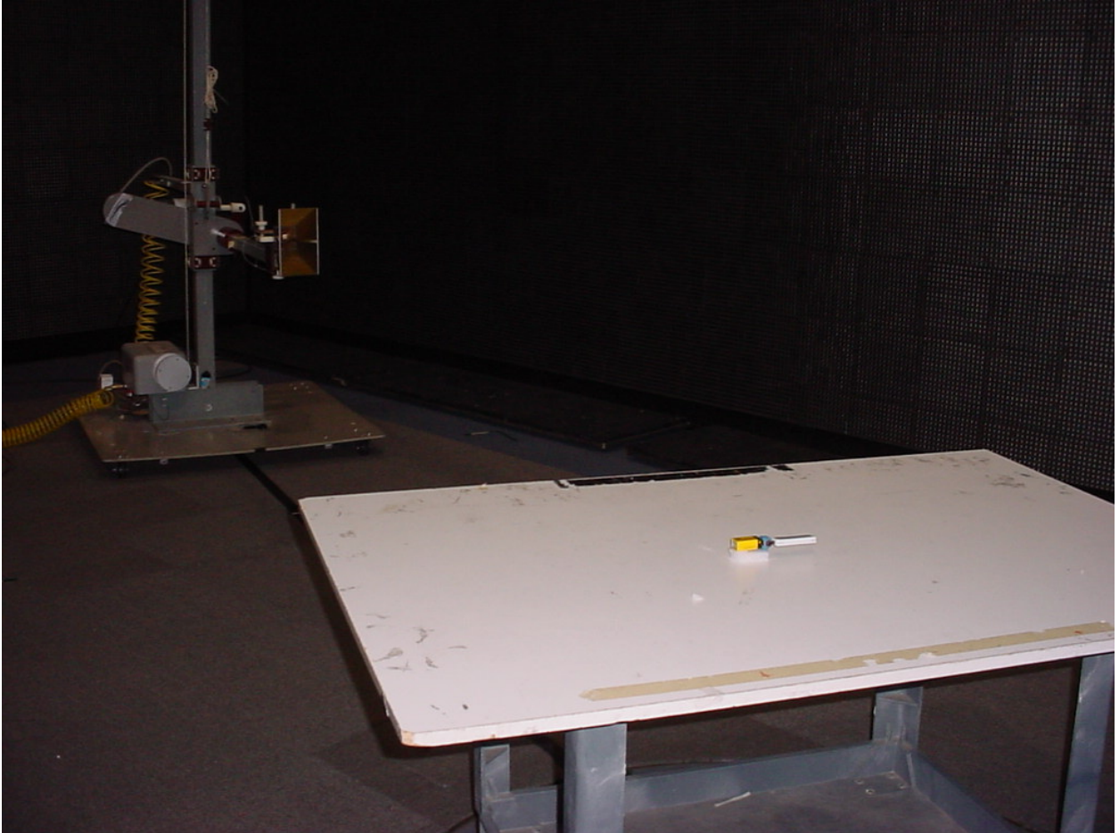
Figure 6: Test Setup Radiated Emissions - Intentional
