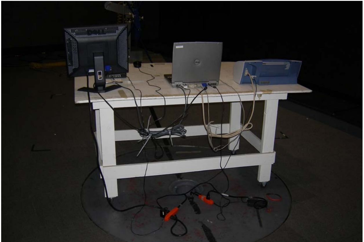
Figure 3: Test Setup Radiated Emissions – Unintentional
