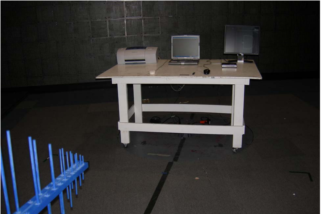
Figure 4: Test Setup Radiated Emissions – Unintentional
