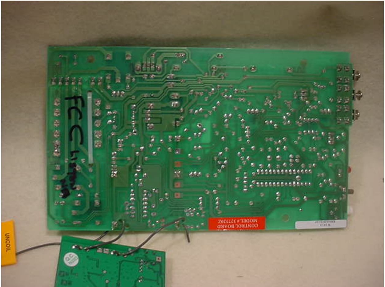
Figure 3: Internal Photographs - Motor Control Board Back
