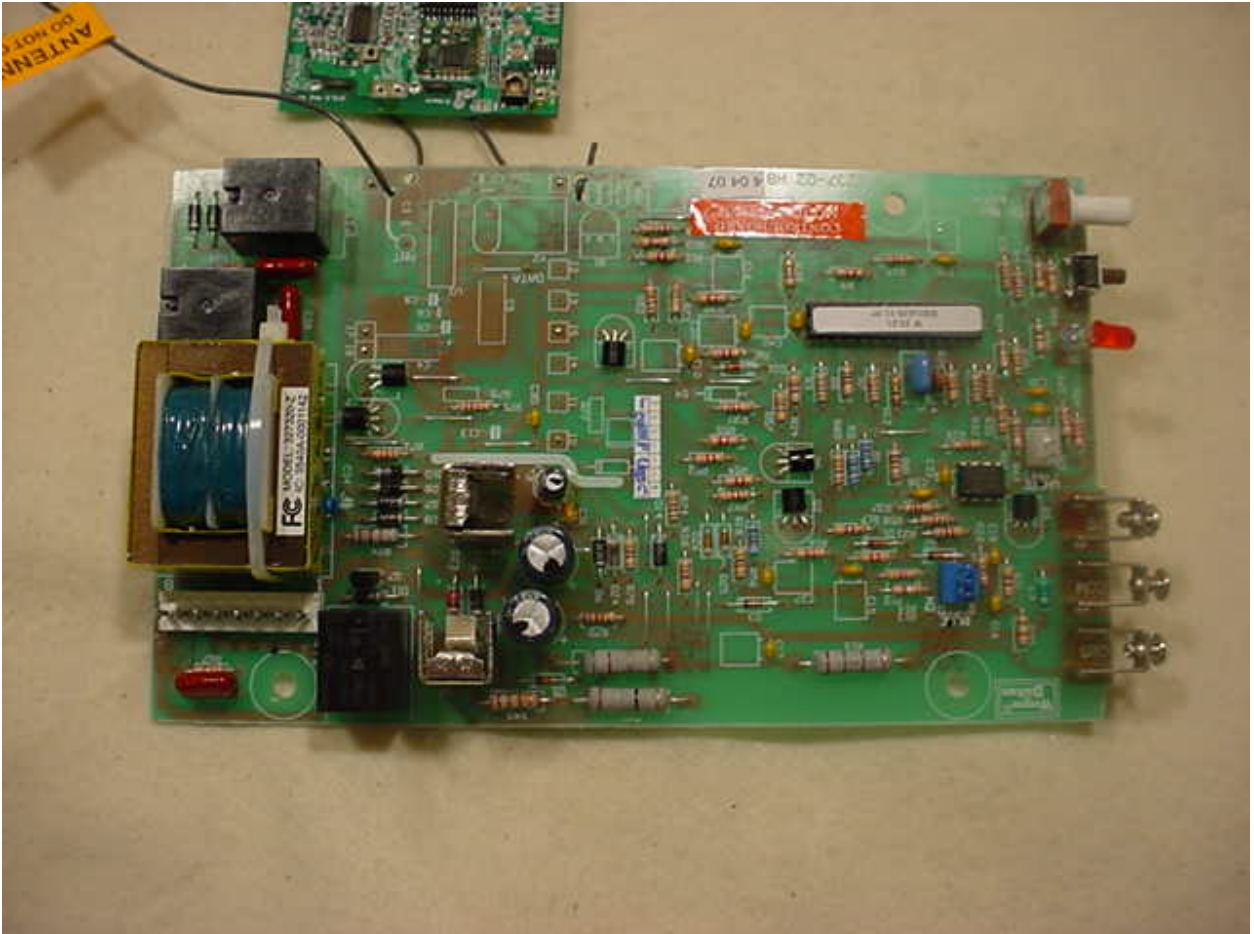
Figure 2: Internal Photographs – Motor Control Board Front
