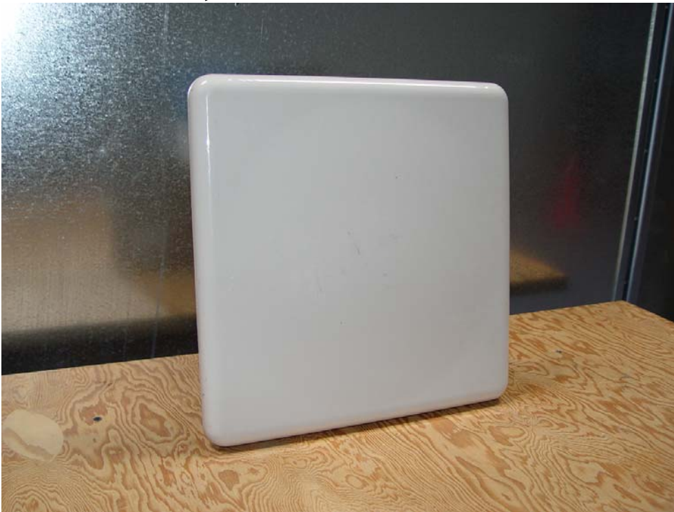
Antenna 9: 5.8GHz, 23 dBi Panel
