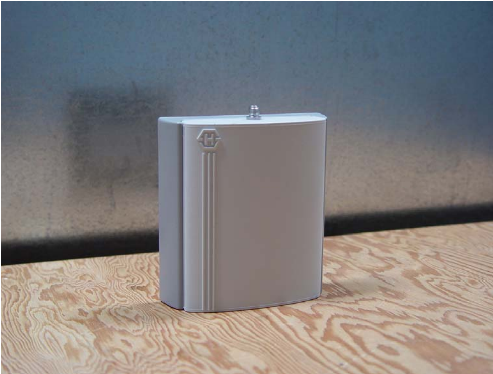
Antenna 1: 2.4GHz, 8 dBi Patch
