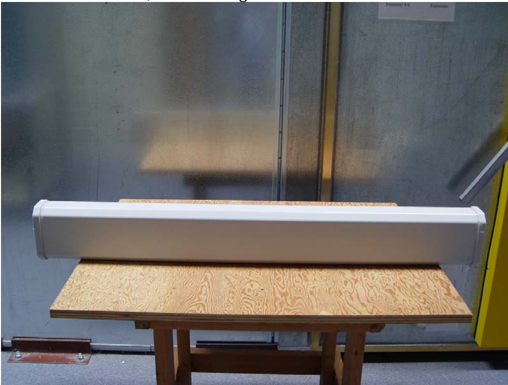
Antenna 4: 2.4GHz, 16 dBi 90 degree Sector
