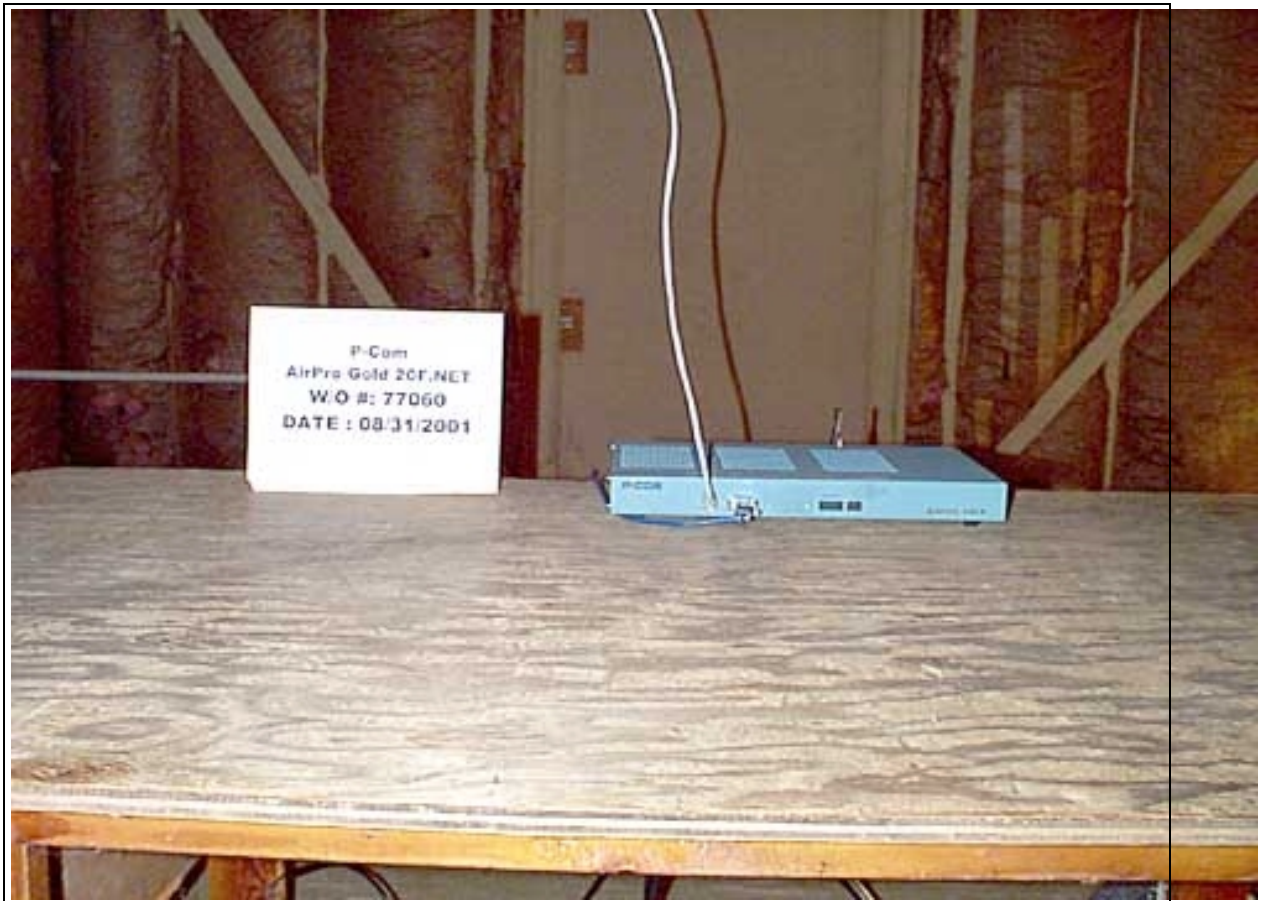
Radiated Emissions - Front View
