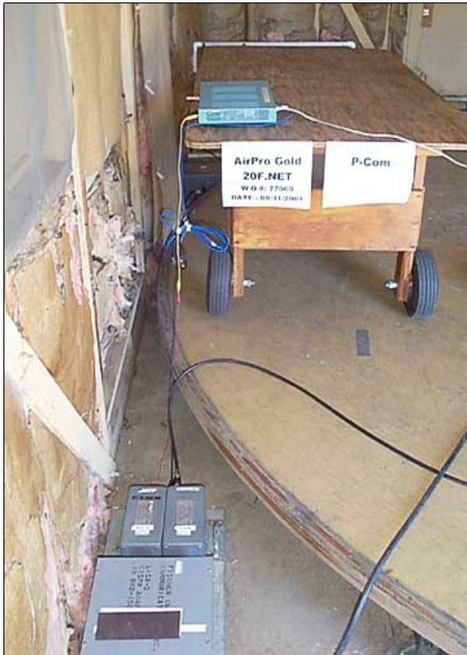
AC Conducted Emissions - Side View
