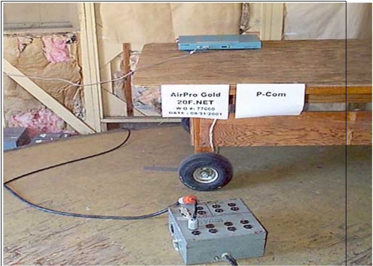
AC Conducted Emissions - Front View
