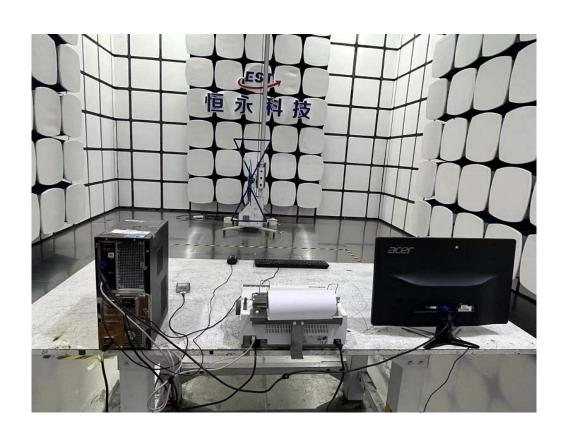
**Radiated Emission Test (Above 1GHz)**
