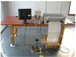
Conducted emission at mains port [Serial mode]
