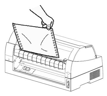
Tearing off continuous forms (front feed)
