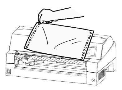
Tearing off continuous forms (rear feed)
