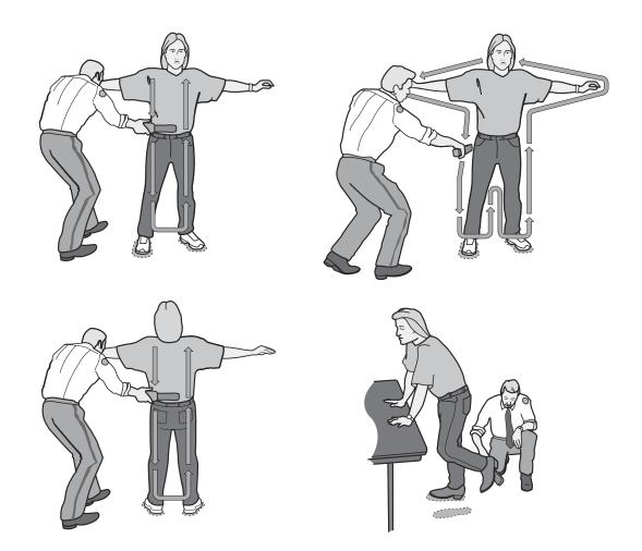
This is an example of procedures for using a handheld metal detector that has at least a 10-inch zone of direction.
