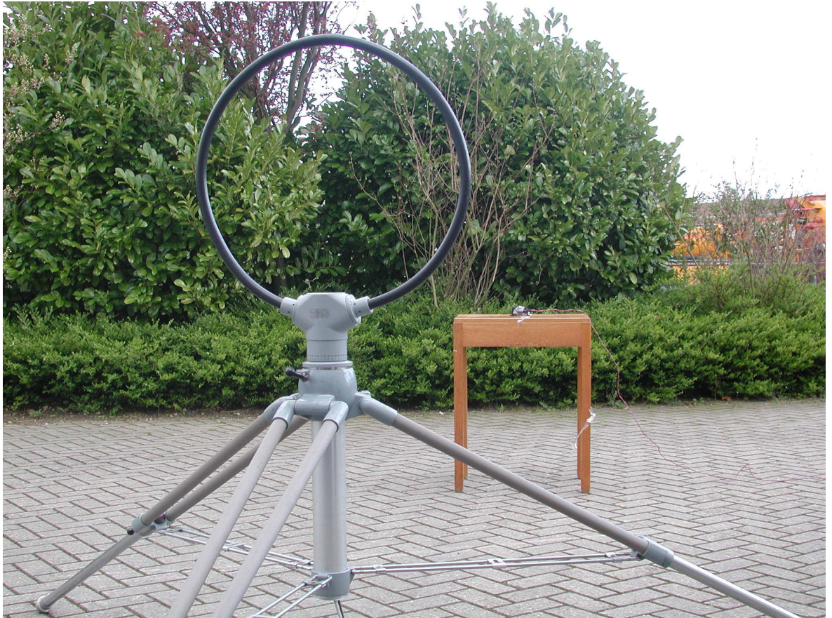
Photograph 5: 3 m test set up, ( < 30 MHz)
