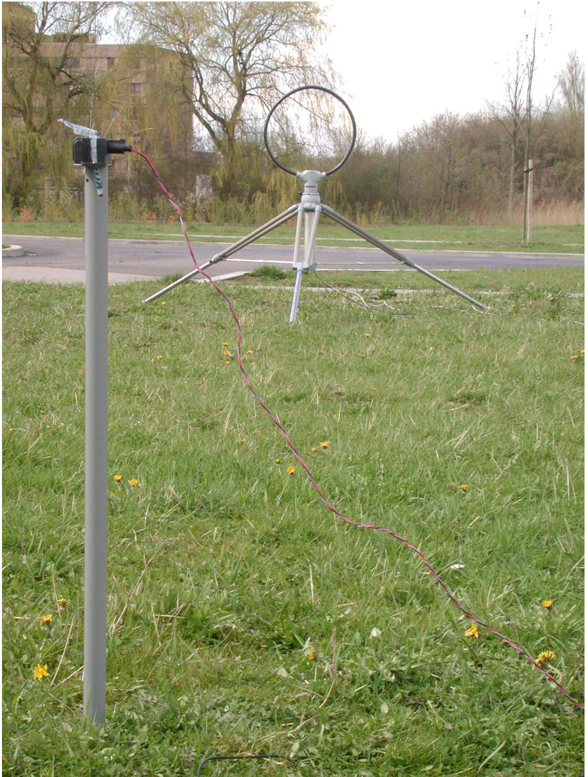
Photograph 4: 10 m test set up, ( < 30 MHz)
