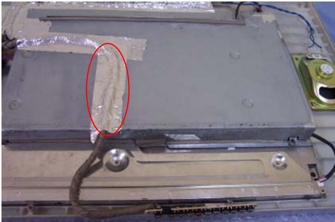
6.Cable of keystroke is shielded and contact case.
