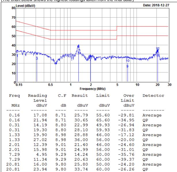
REMARKS: 1. Level (dBuV) = Read Level (dBuV) + LISN Factor (dB) + Cable Loss (dB)
