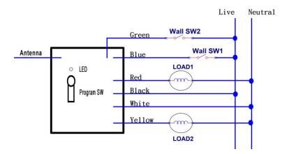
For "Inclusion" in (adding to) a network: Put the Z-Wave™ Interface Controller into "inclusion" mode, and following its instruction to add the ZL 7432 to your controller. To get in the "inclusion" mode, the distance between module and controller is suggested to be in one meter. Turn on and turn off the wall switch that connects with ZL 7432 module 4 times to be included. (or press the Program SW 4 times within 2 seconds to be included)
