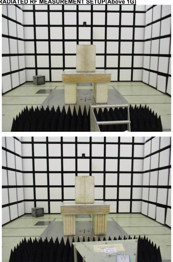
**RADIATED RF MEASUREMENT SETUP(Above 1G)**
