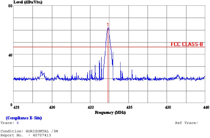
Report No. : 40707413 Test Engr. : ALEX PAN Company : Vision Automobile Electronics Industrial Co., Ltd. EUT : PPRF64/128 Test Config : EUT / ALL PERIPHERALS Type of Test: FCC CLASS B Mode of Op. : RX MODE
