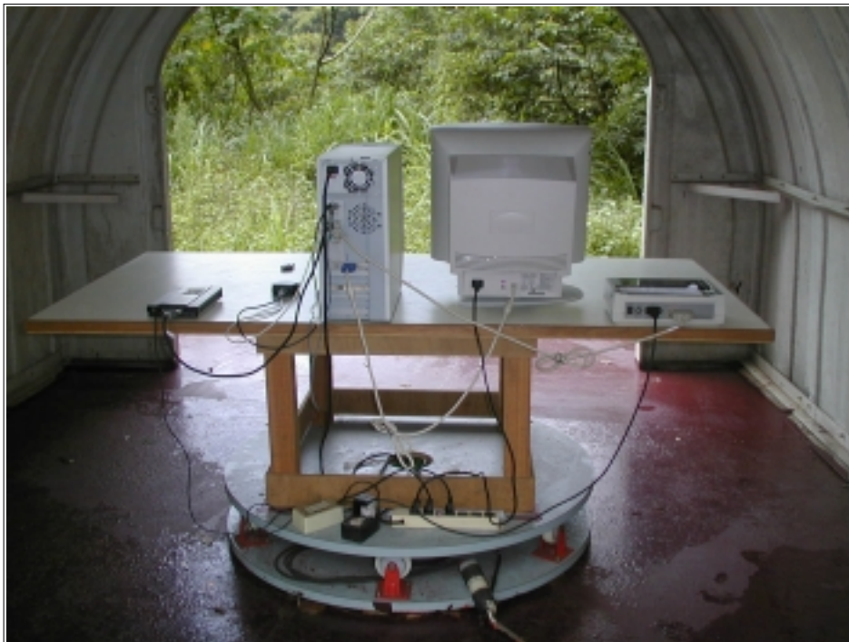
Radiated Emission Setup Photos (Worst Emission Position)
