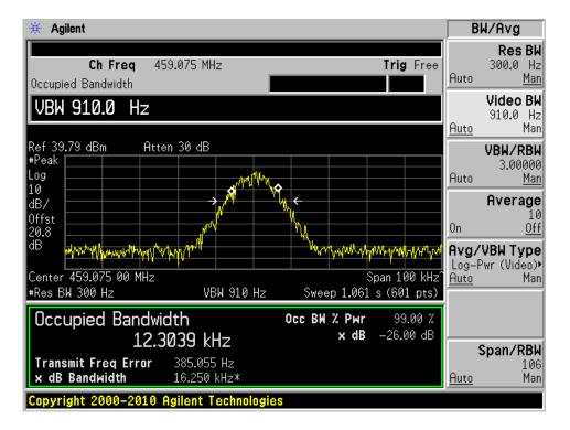
GMSK, Data Rate: 19200bps, 25 kHz Channel Space, Middle Channel – 459.075 MHz
