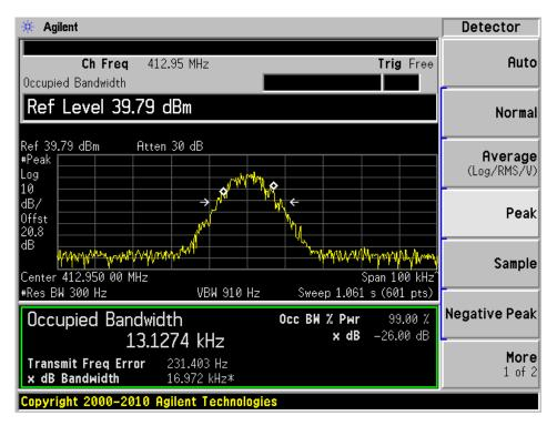
GMSK, Data Rate: 19200 bps, 25 kHz Channel Space, Middle Channel – 412.95 MHz
