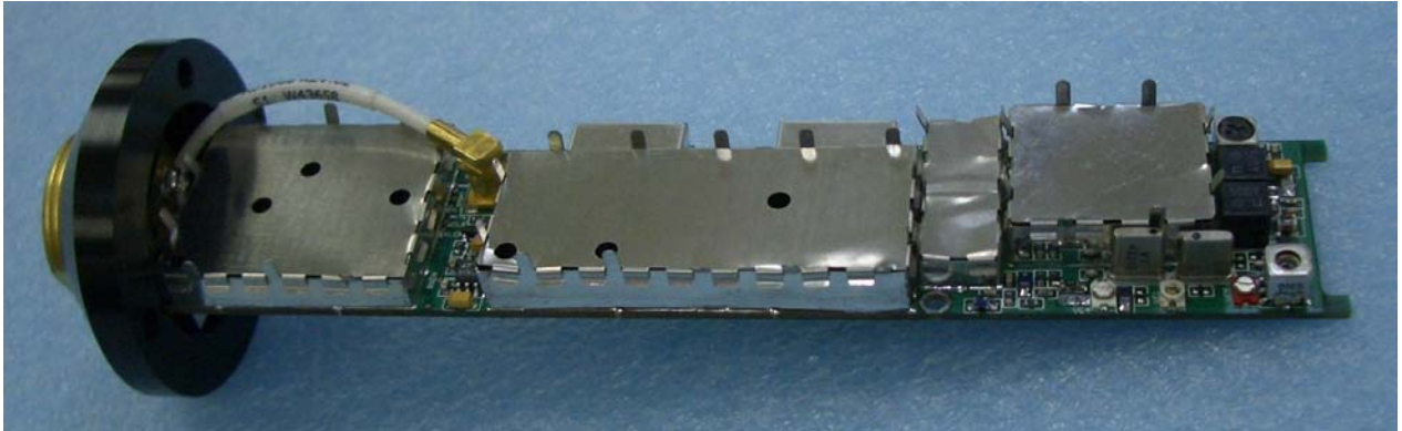
EUT – Radio PCB Top View with Shielding
