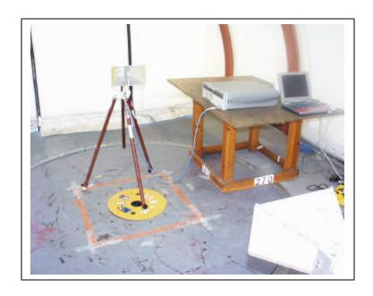
**Substitution Method Above 1GHz Setup Photo**
