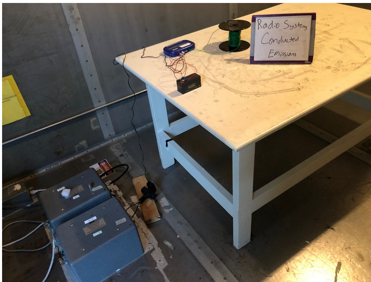
Figure 7. Powerline Conducted Emissions Test Configuration
