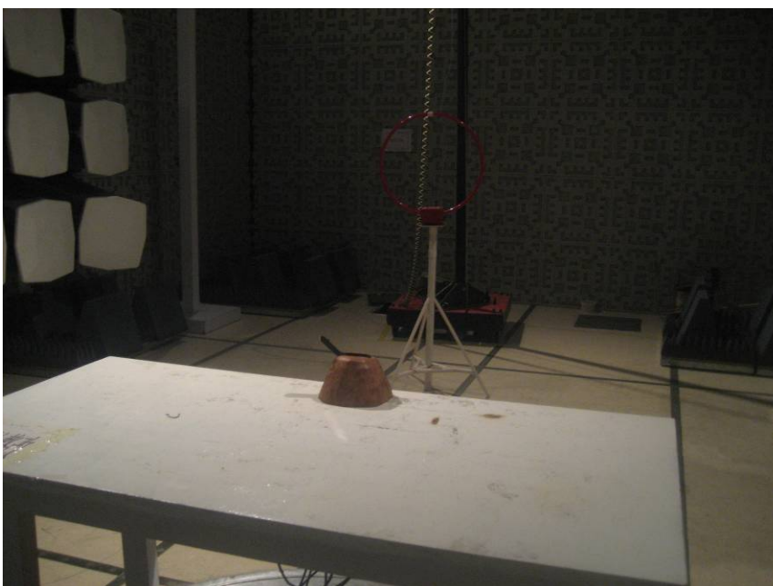
TEST SETUP OF RADIATED EMISSION ( \leq 30 MHz Loop Antenna)
