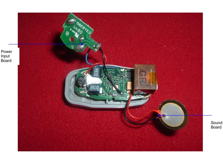
5.5 Top View of EUT Cover removed Host Board, Sound Board, and Power Input Board
