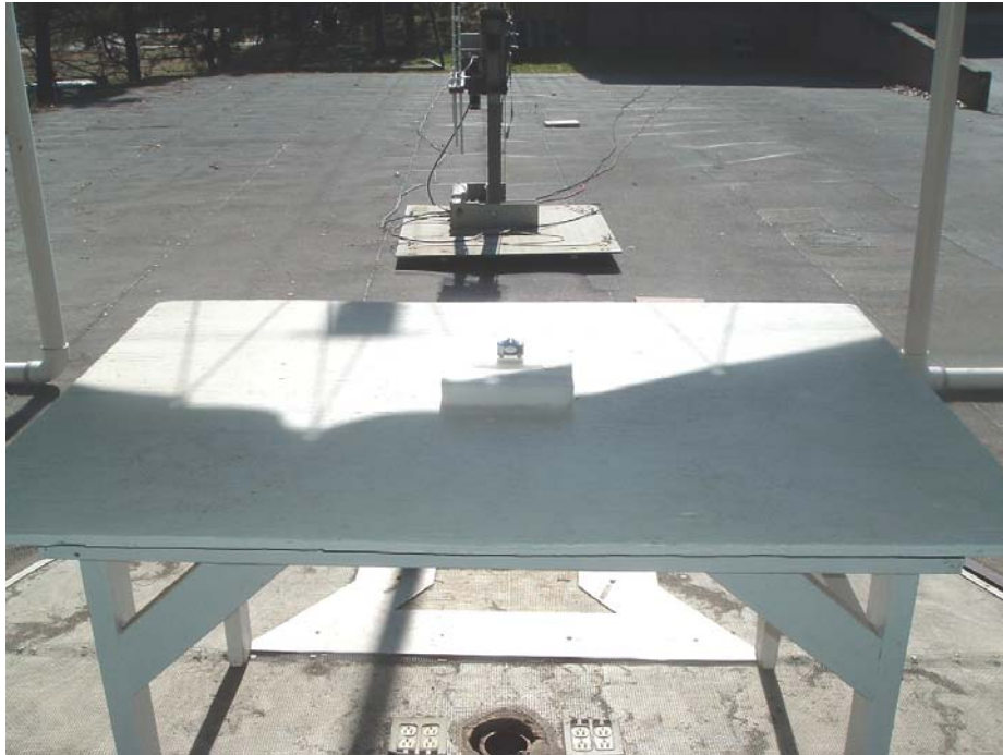
5.9 Radiated Emissions Rear View of Test Setup
