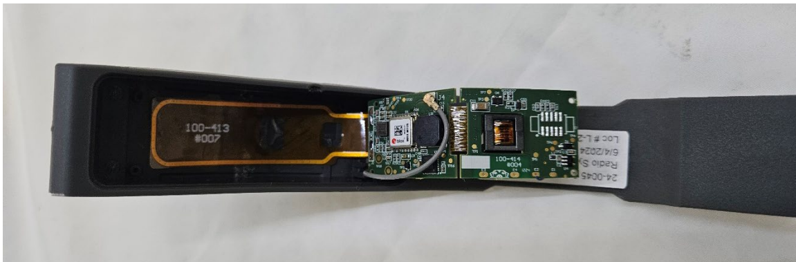
Figure 4. Main PCB Back and Antenna
