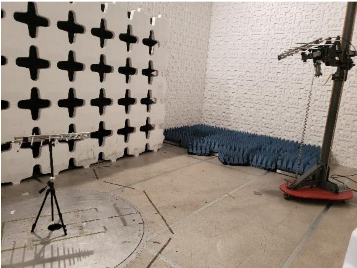
Figure 8. Substitution Test Setup, 200 MHz to 1 GHz
