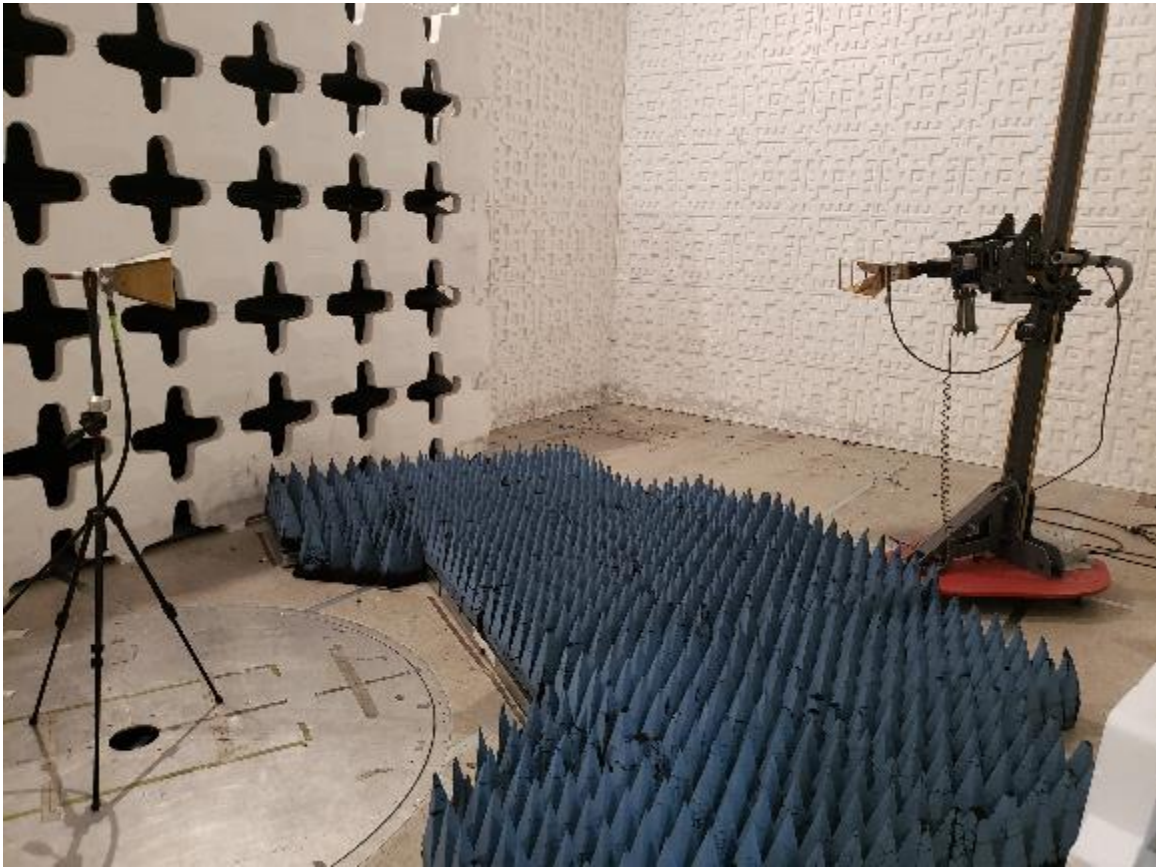
Figure 9. Substitution Test Setup, Above 1 GHz
