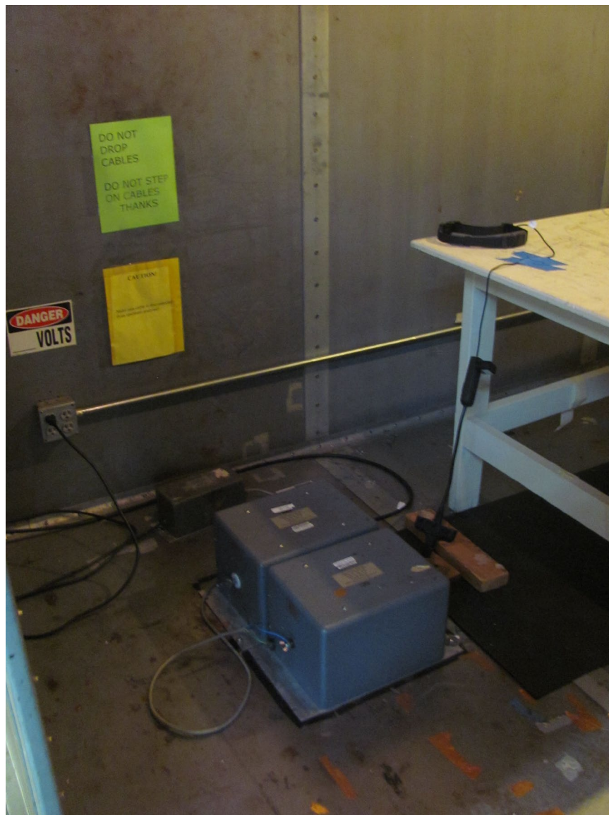
Figure 6. Conducted Emissions Test Setup
