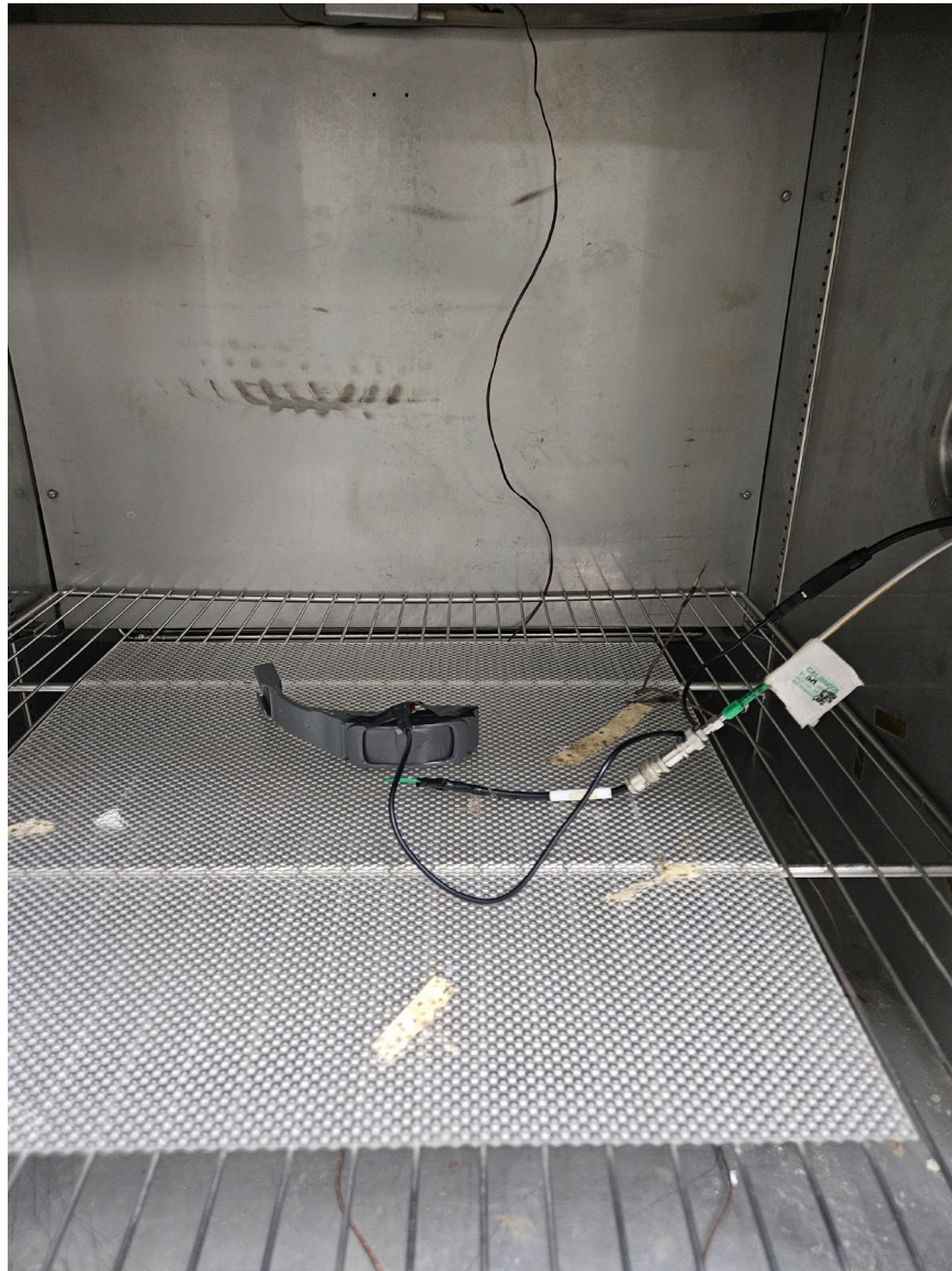
Figure 10. Frequency Stability Test Setup
