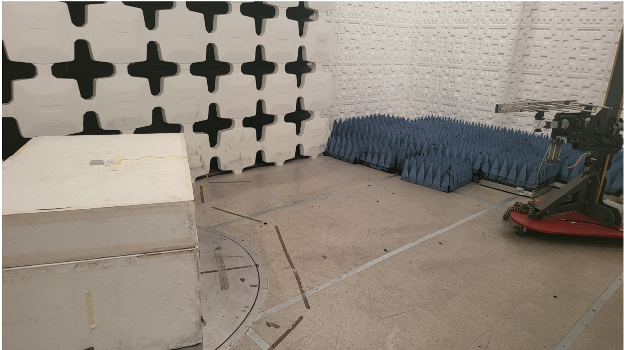
Figure 4. Radiated Emissions Test Setup, 200 MHz to 1 GHz
