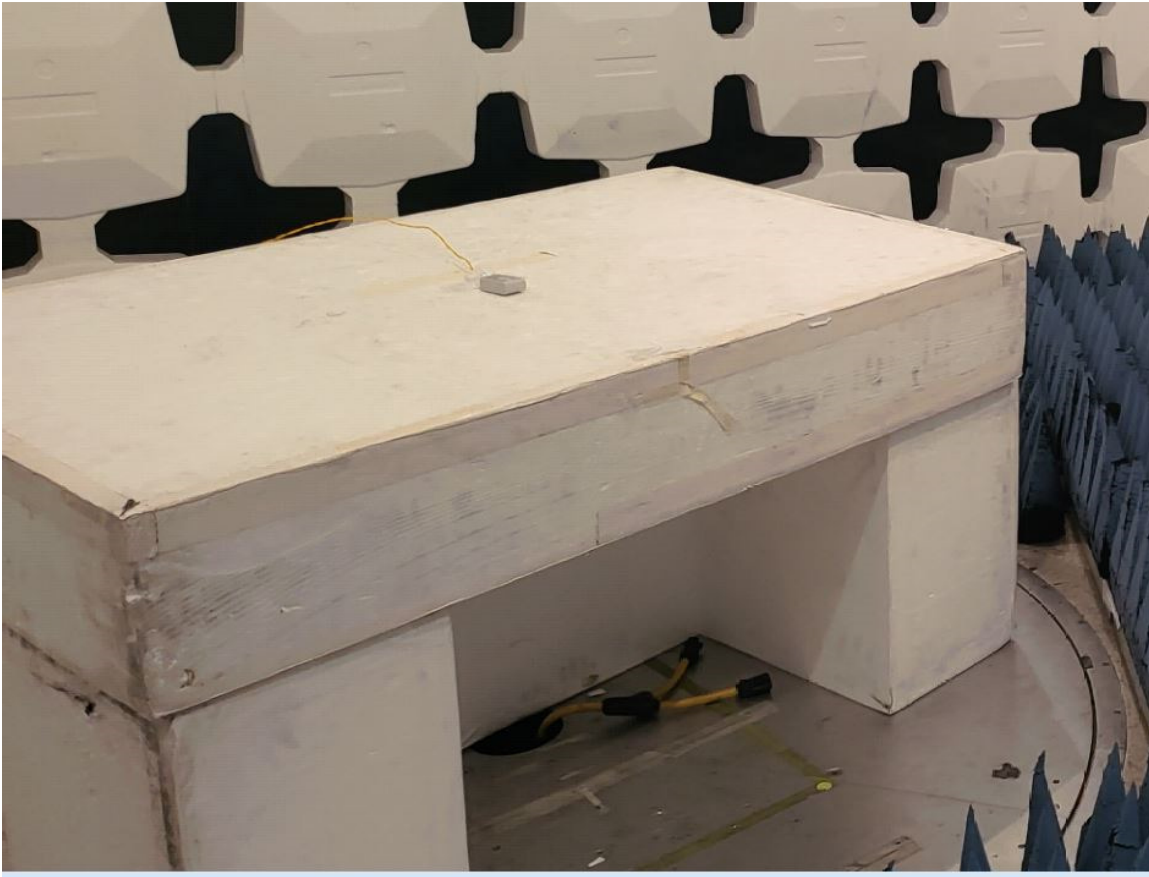
Figure 1. Radiated Emissions Test Setup
