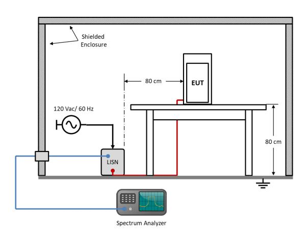
Figure 3. EUT Test Configuration - AC Power Line Conducted Emissions
