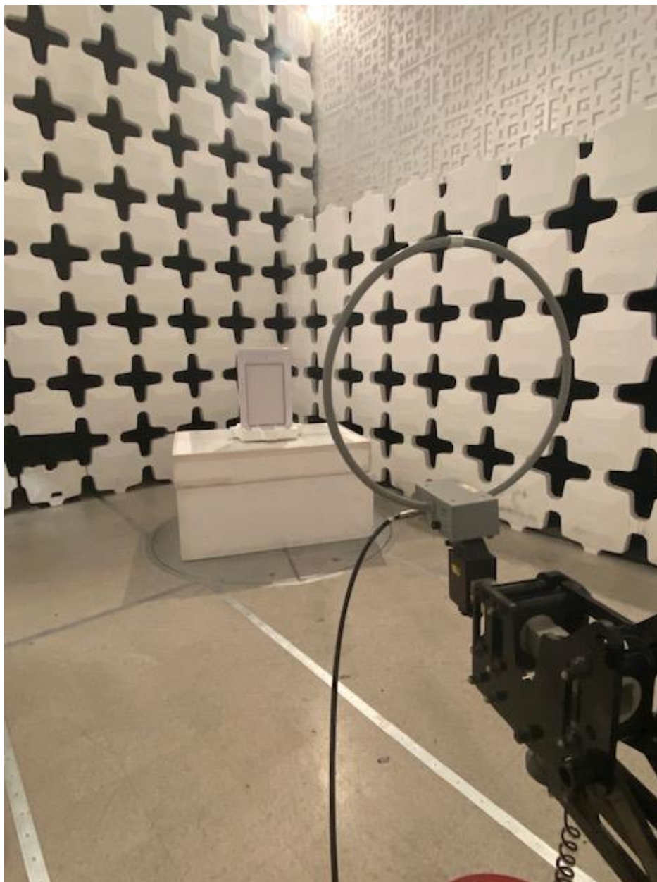
Figure 2. Radiated Emissions Test Setup, 9 kHz to 30 MHz
