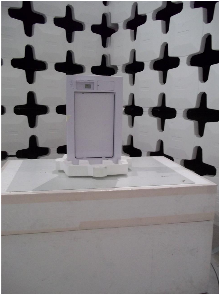
Figure 1. Radiated Emissions Test Setup
