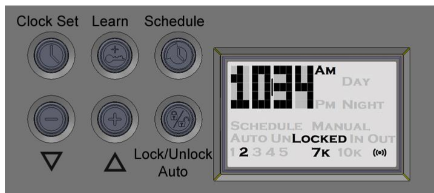
Figure 1: Pushbuttons for Controlling Door Functionality
