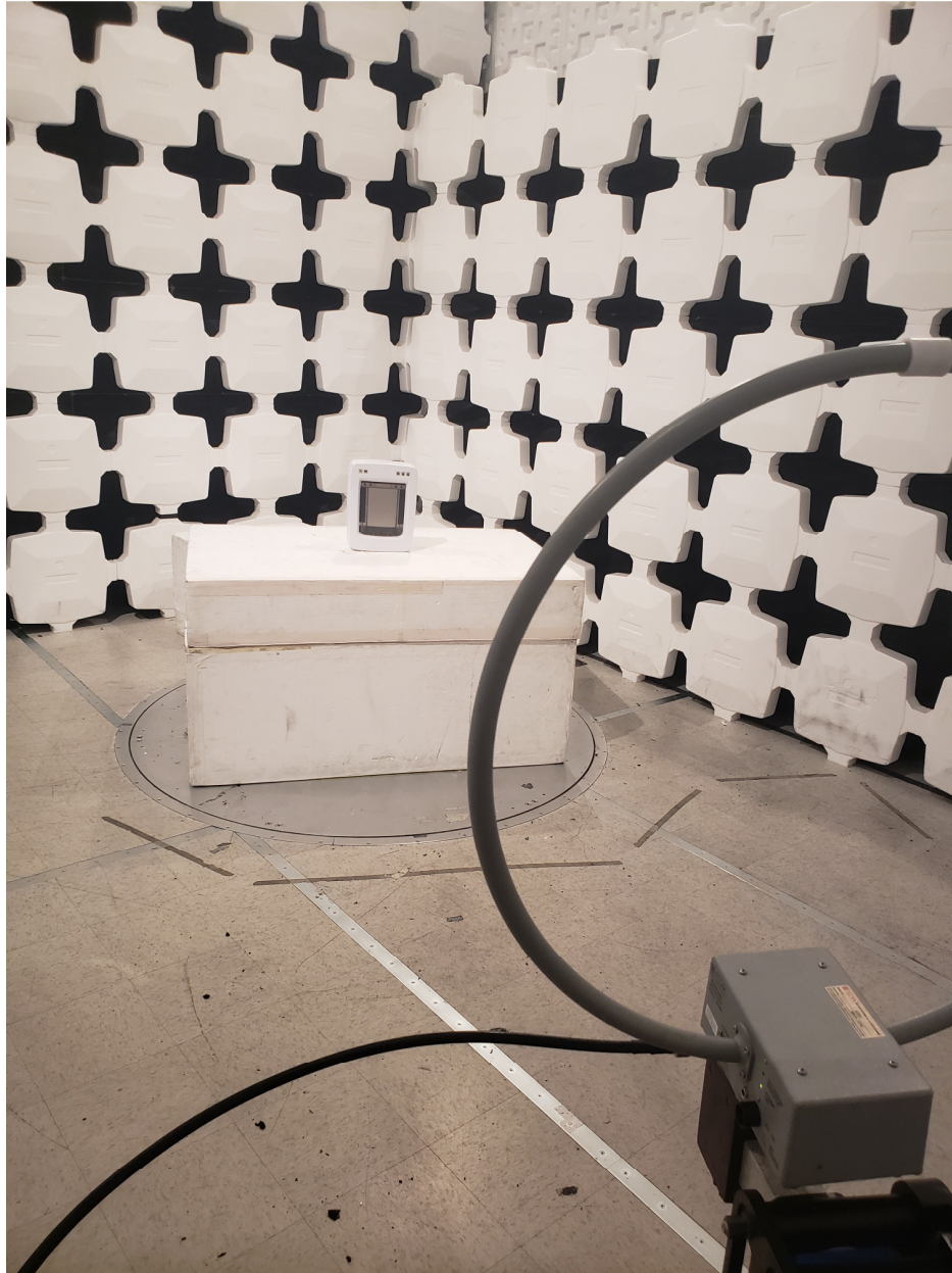
Figure 2. Radiated Emissions Test Setup, 9 kHz to 30 MHz
