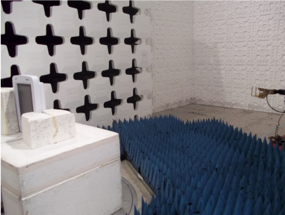
Figure 5. Radiated Emission Test Setup, above 1 GHz
