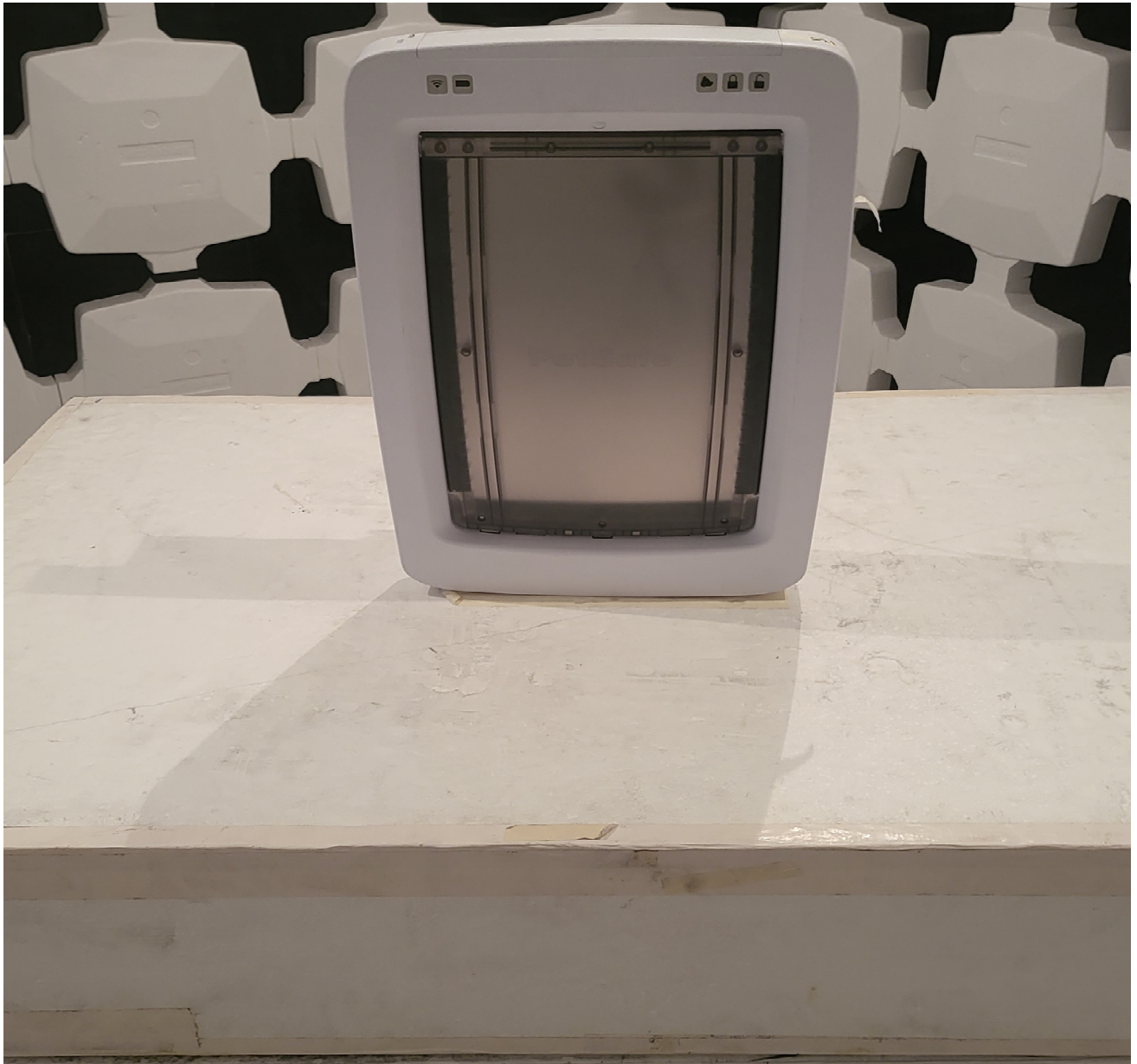
Figure 1. Radiated Emissions Test Setup
