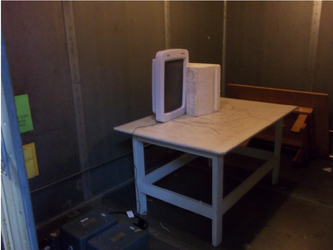
Figure 6. Powerline Conducted Emission Test Setup
