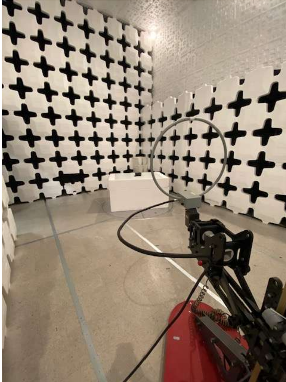
Figure 7. Radiated Emissions Test Setup (Below 30 MHz), Model RAC00-16952
