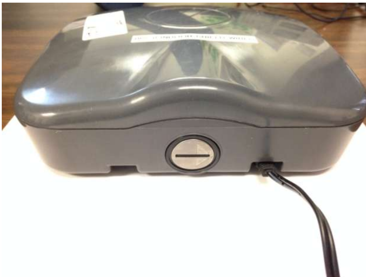
Figure 9. RAC00-16949 and RAC00-16992, Battery and AC/DC Power Adapter Cord Inserted
