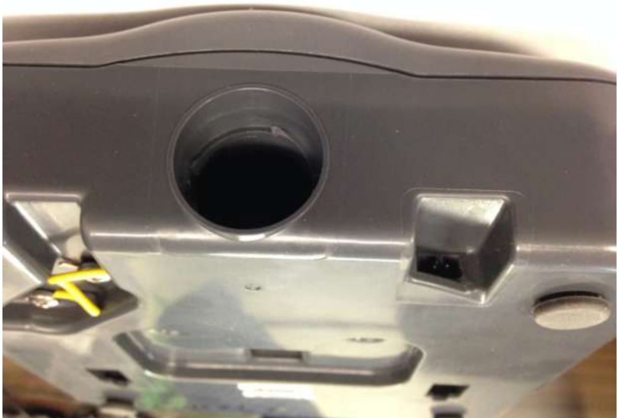
Figure 7. RAC00-16949 and RAC00-16992, Battery Port and AC/DC Input Port
