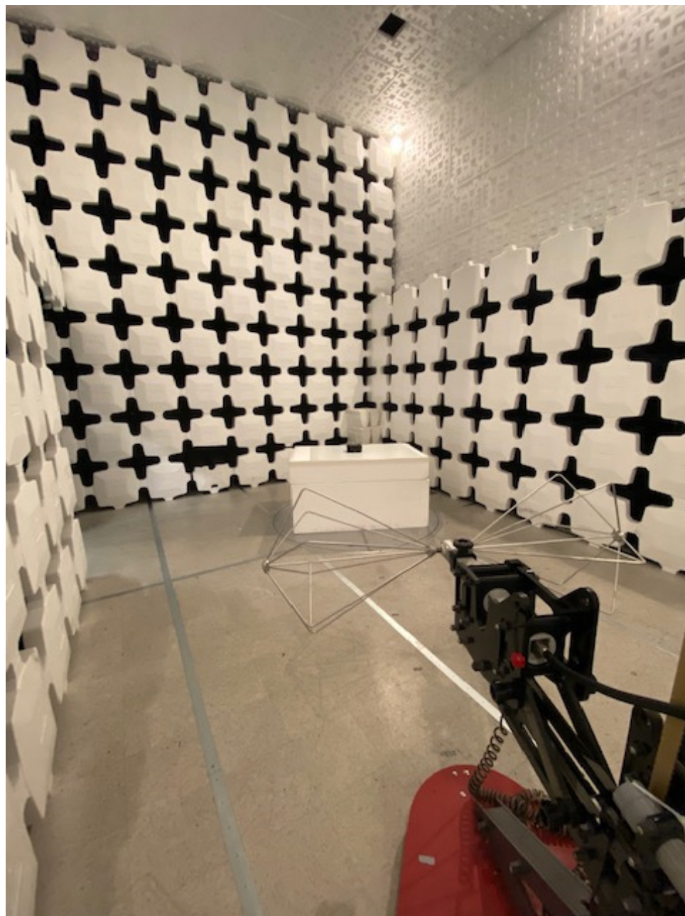
Figure 8. Radiated Emissions Test Setup, 30 MHz to 200 MHz (Radio Test with EUT in worst case position), Outdoor Unit
