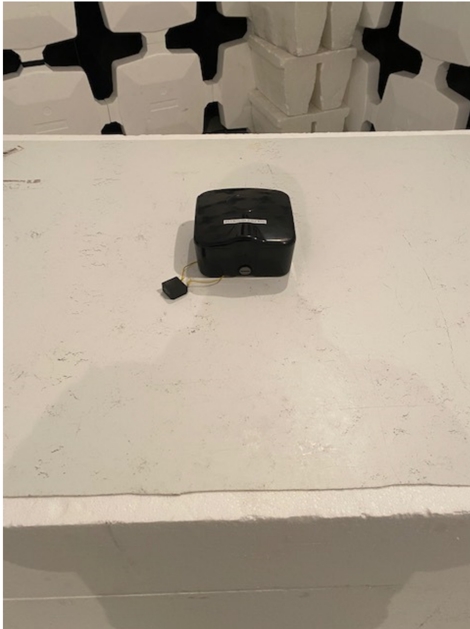
Figure 6. Radiated Emissions Test Setup, Close-Up, Outdoor Unit
