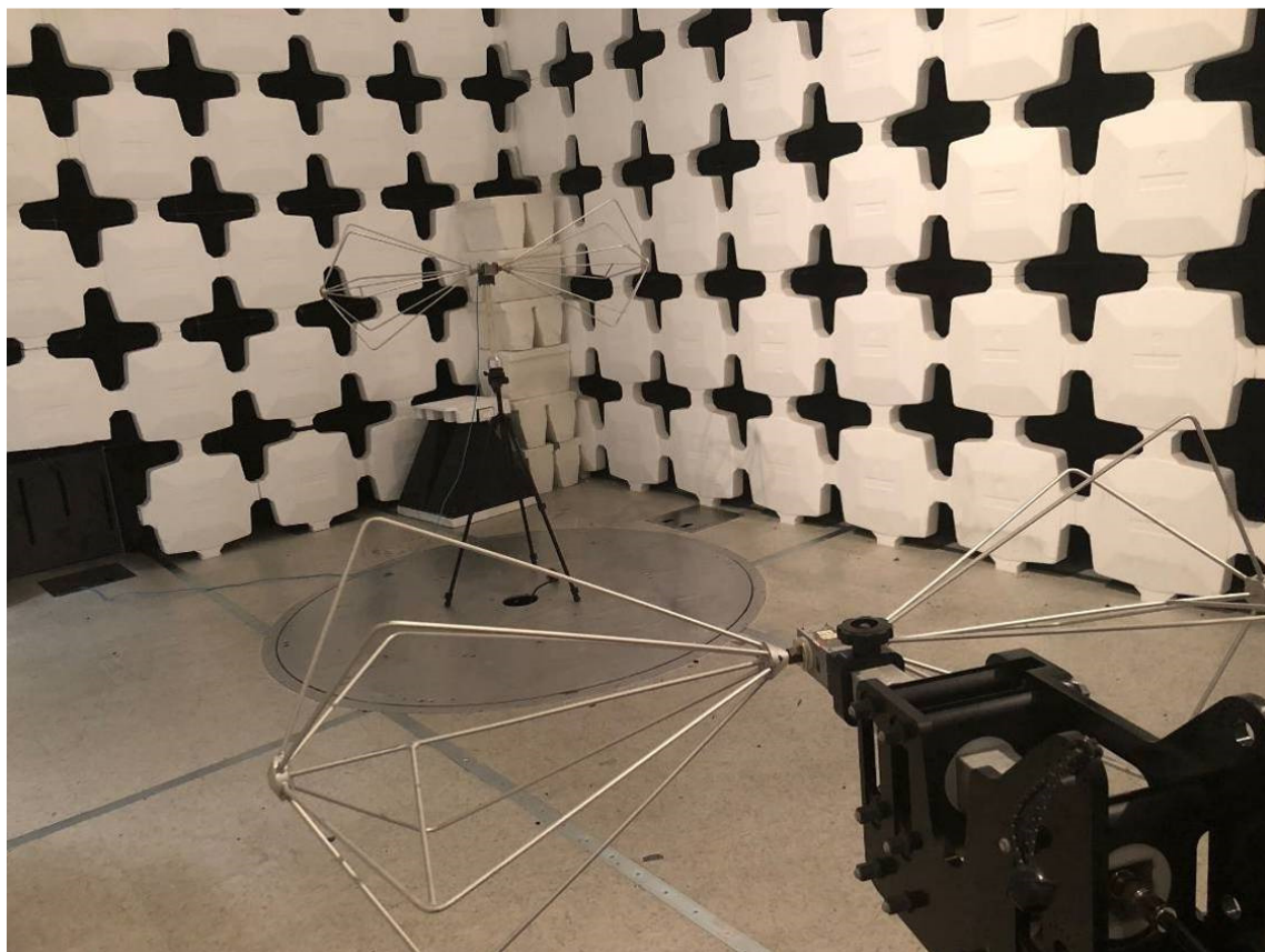
Figure 15. Substitution Testing 30-200 MHz
