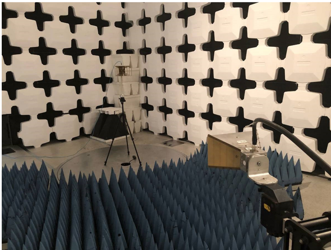
Figure 17. Substitution Testing above 1 GHz
