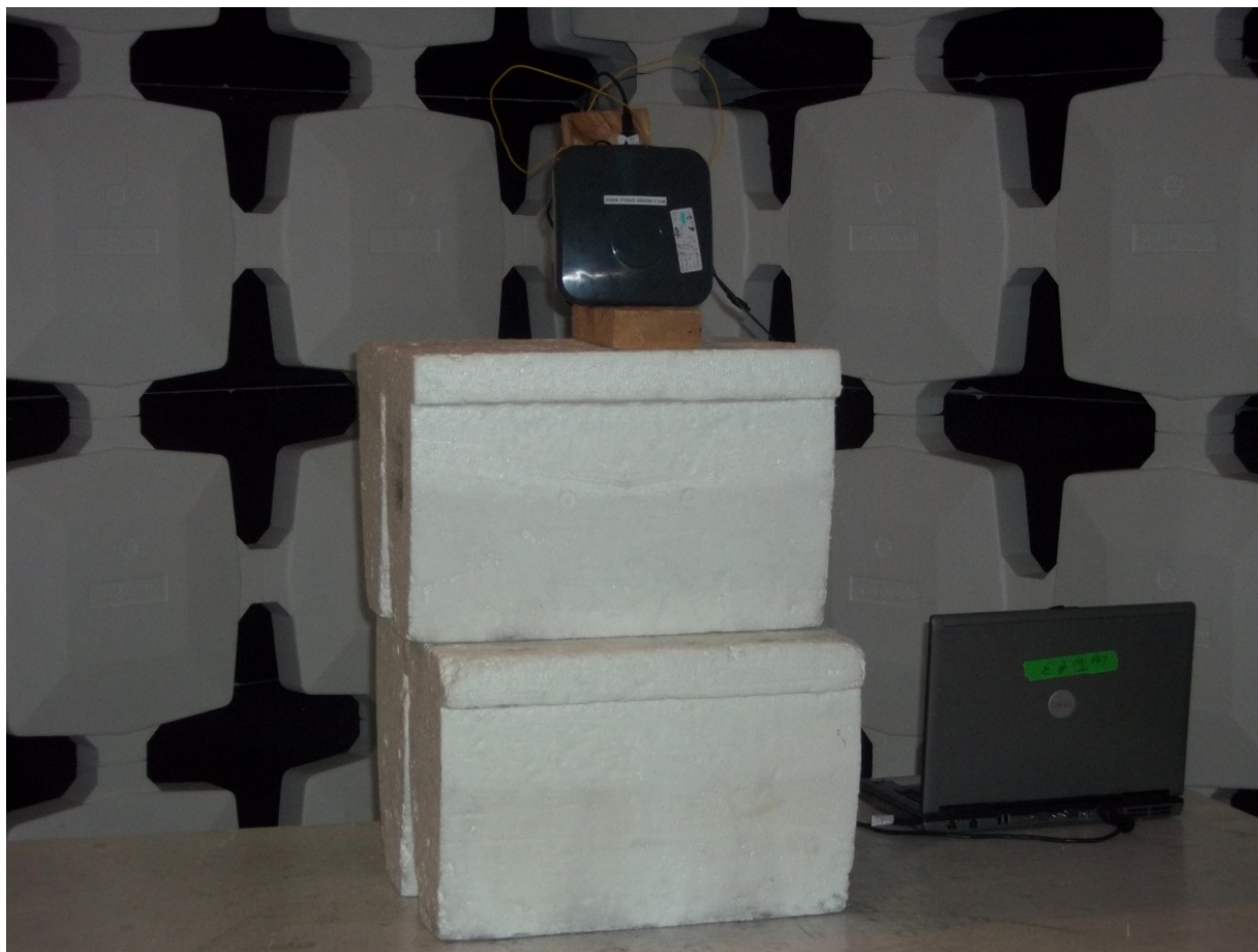
Figure 11. EUT above 1 GHz Test Configuration (Intentional Emissions)
