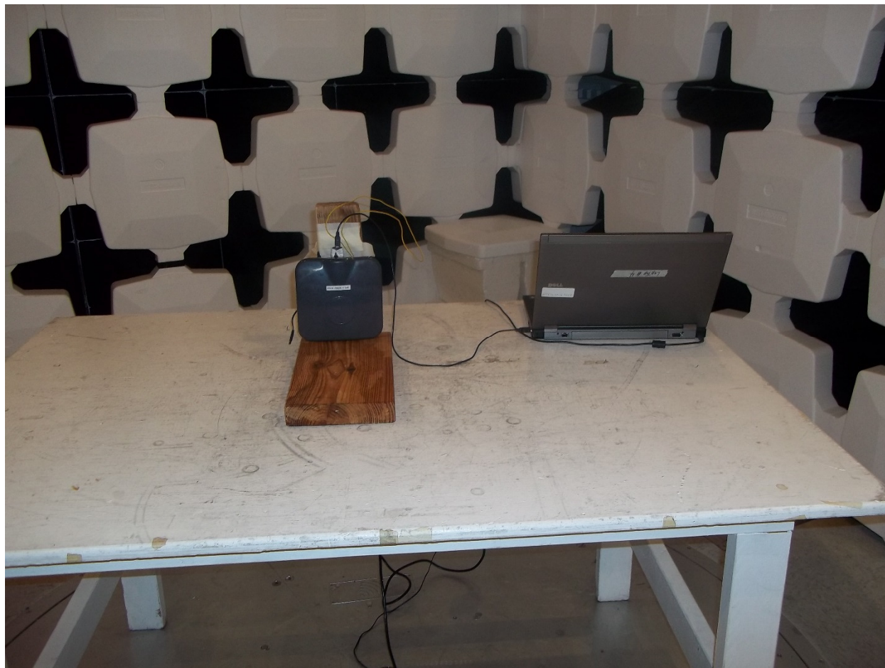
Figure 1. Radiated Emissions Test Setup, Close-Up, Indoor Unit
