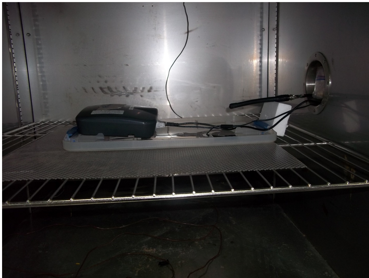
Figure 13. Frequency Stability Test Setup
