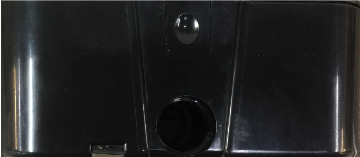
Figure 14. RAC00-16953, Battery Port and AC/DC Input Port
