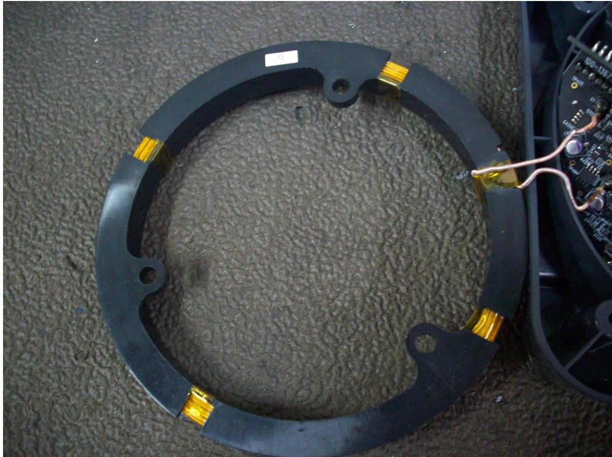
Figure 7. Top of Coil Attached to the PCB
