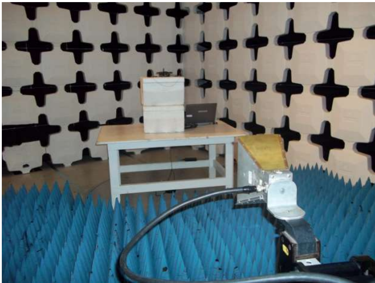
Figure 6. EUT above 1 GHz Test Configuration (Intentional Emissions)
