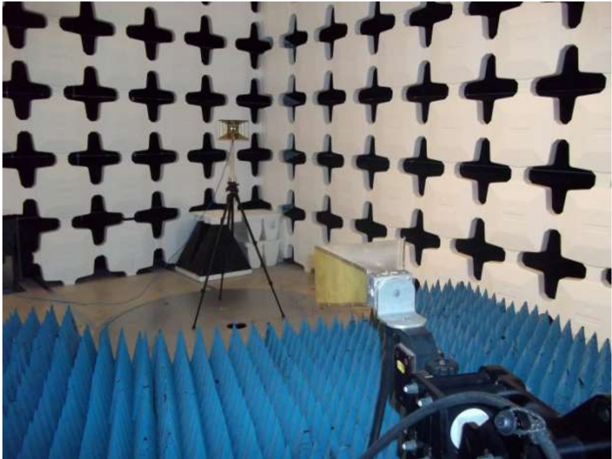
Figure 11. Substitution Testing above 1 GHz
