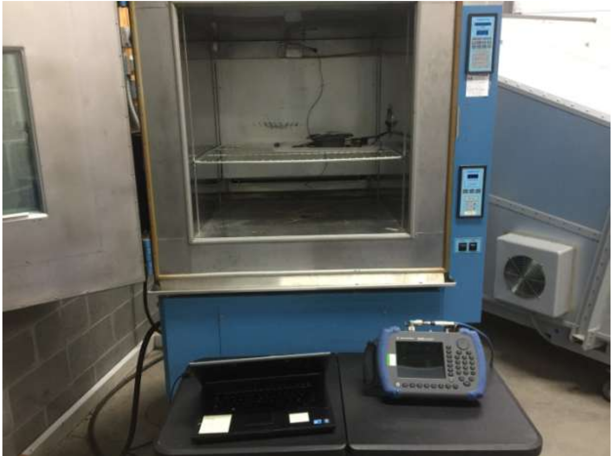
Figure 7. Frequency Stability Test Setup
