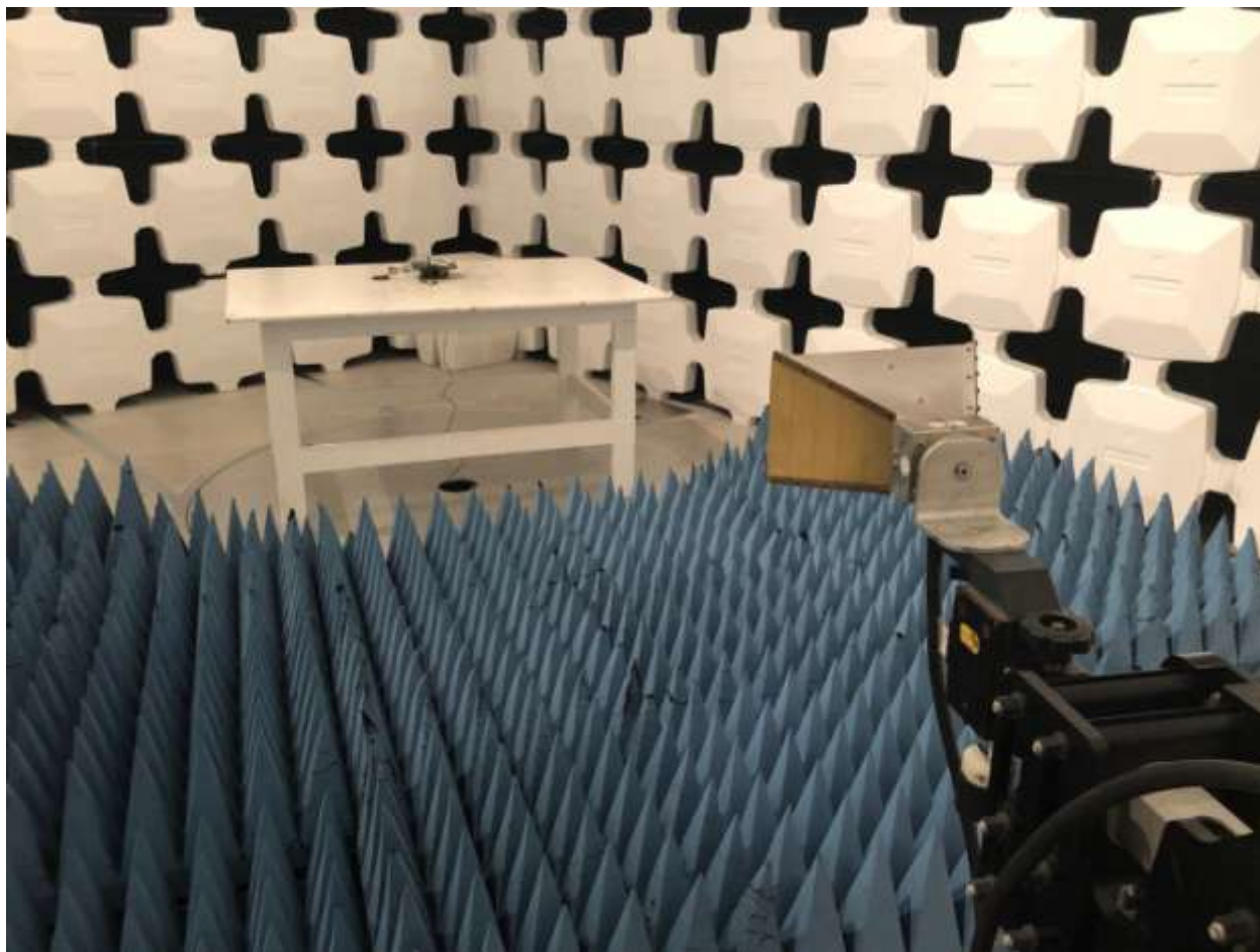
Figure 5. Radiated Emissions Test Setup, Above 1 GHz (Radio Test with EUT in worst case position)
