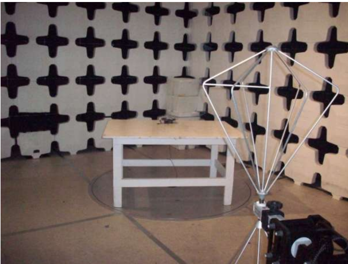
Figure 3. Radiated Emissions Test Setup, 30 MHz to 200 MHz (Radio Test with EUT in worst case position)
