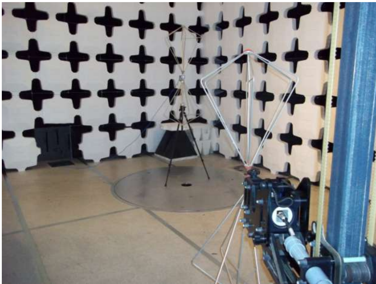
Figure 9. Substitution Testing 30-200 MHz
