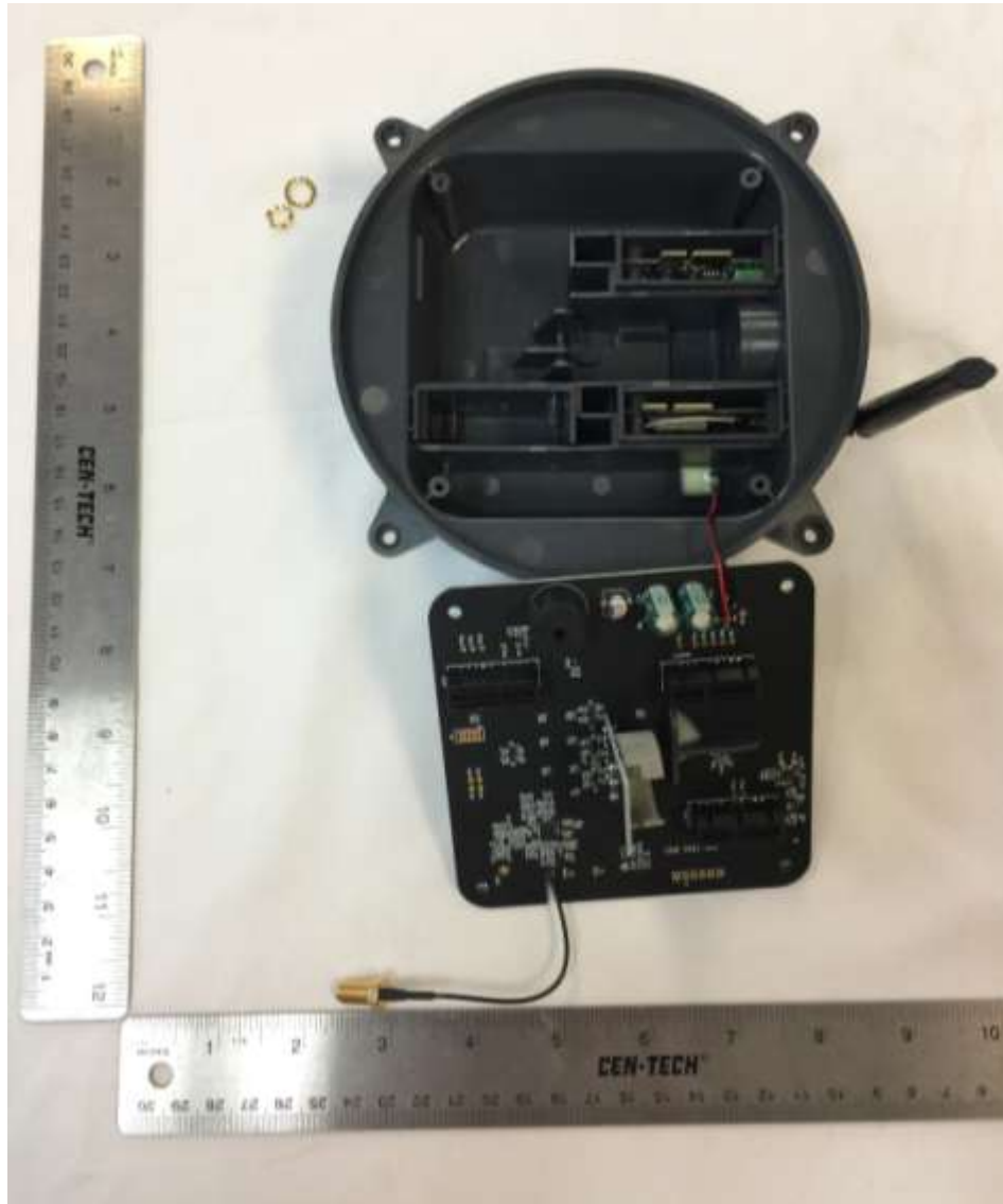
Figure 3. EUT with PCB Removed from Enclosure
