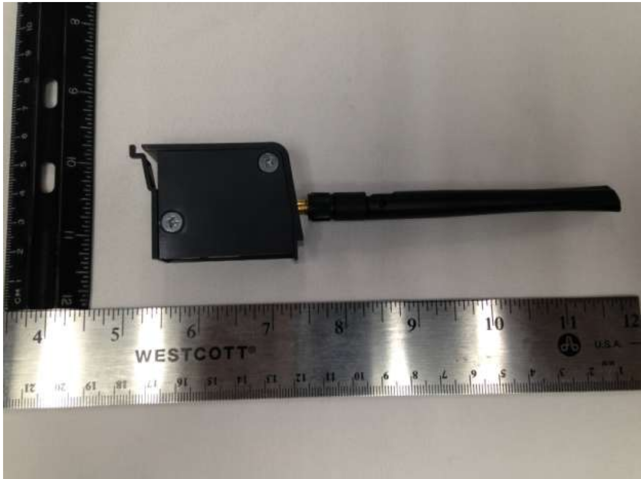
Figure 4. WiFi Module (Pre-Certified) Removed from Main Enclosure
