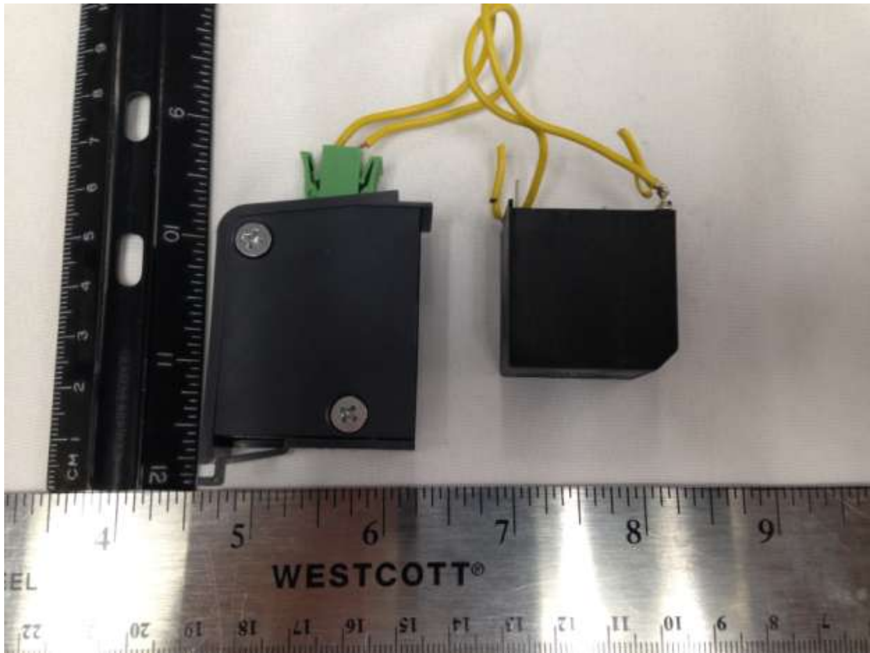
Figure 5. Long Wire Module (Separate Modular Certification Pending) Removed from Main Enclosure
