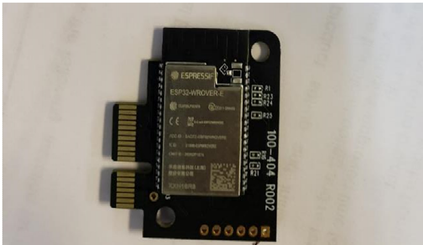
Figure 6. Wi-Fi Module (Pre-Certified) Removed from Enclosure
