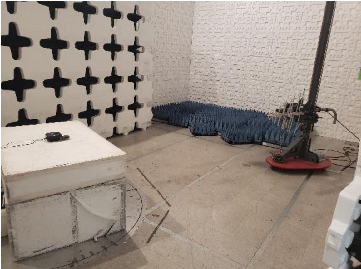
Figure 4. Radiated Emissions Test Setup, 200 MHz to 1GHz, Back
