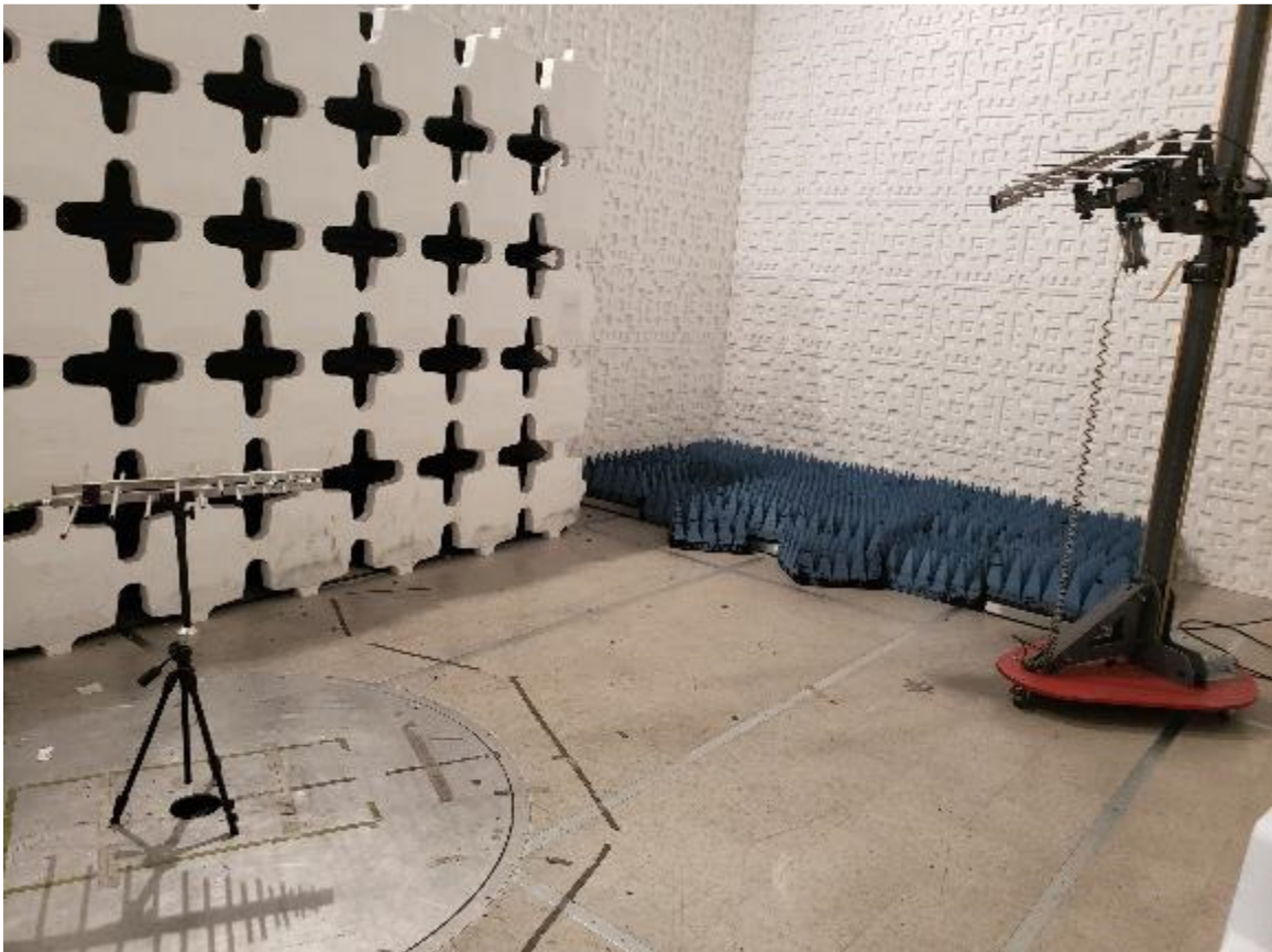
Figure 8. Substitution Test Setup, 200 MHz to 1 GHz
