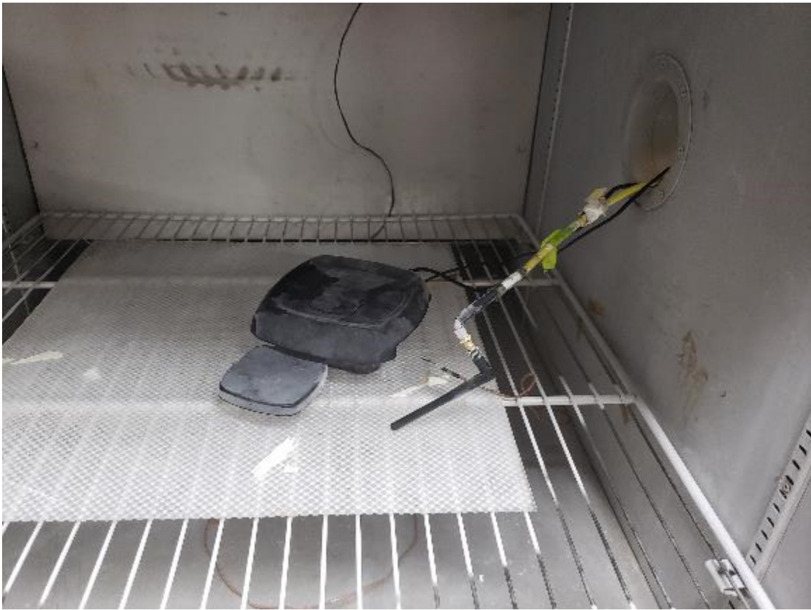
Figure 10. Frequency Stability Test Setup
