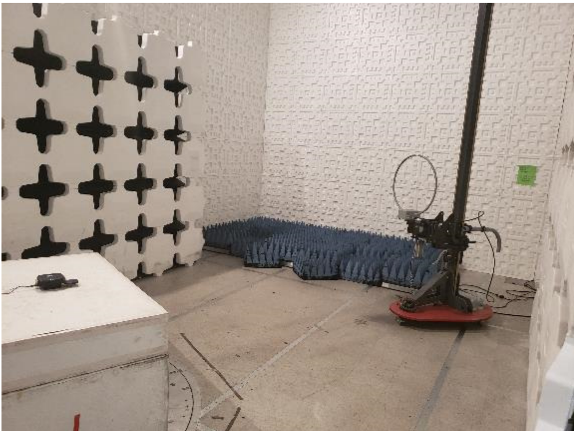
Figure 2. Radiated Emissions Test Setup, .009 MHz to 30 MHz
