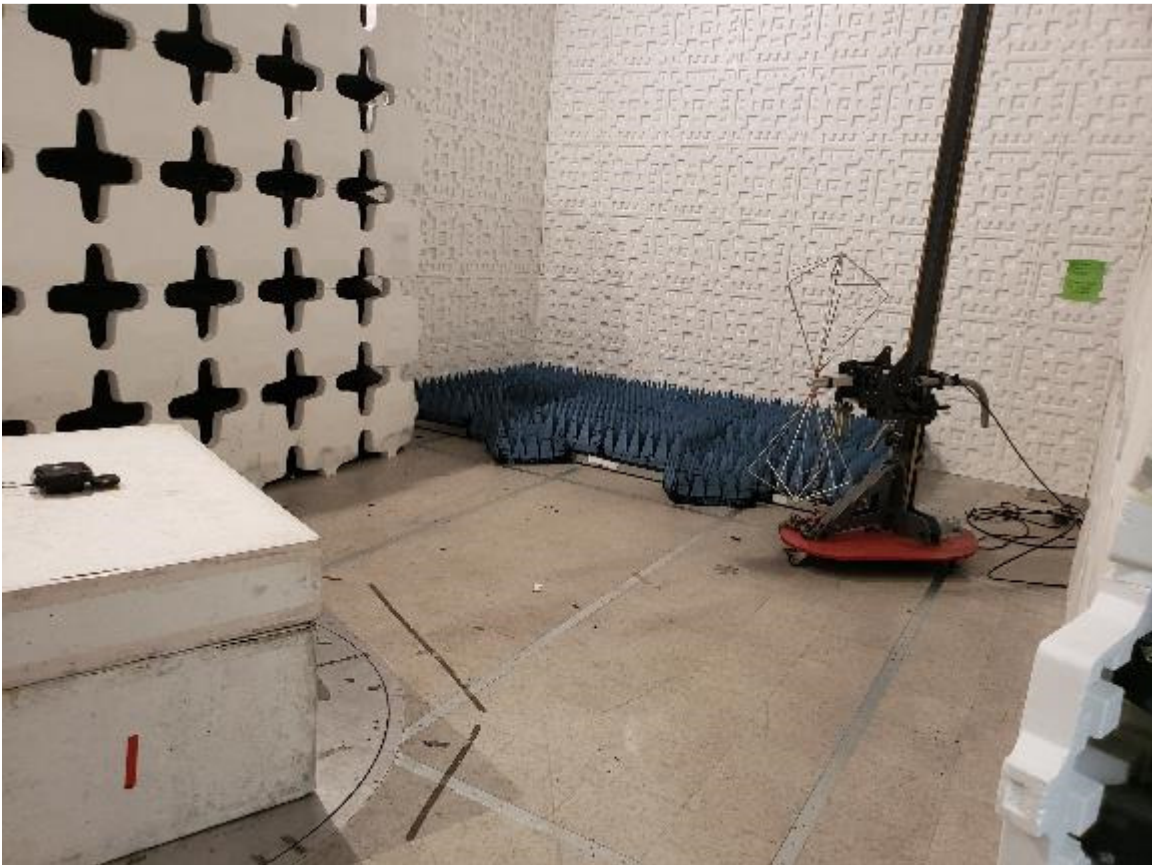
Figure 3. Radiated Emissions Test Setup, 30 MHz to 200 MHz
