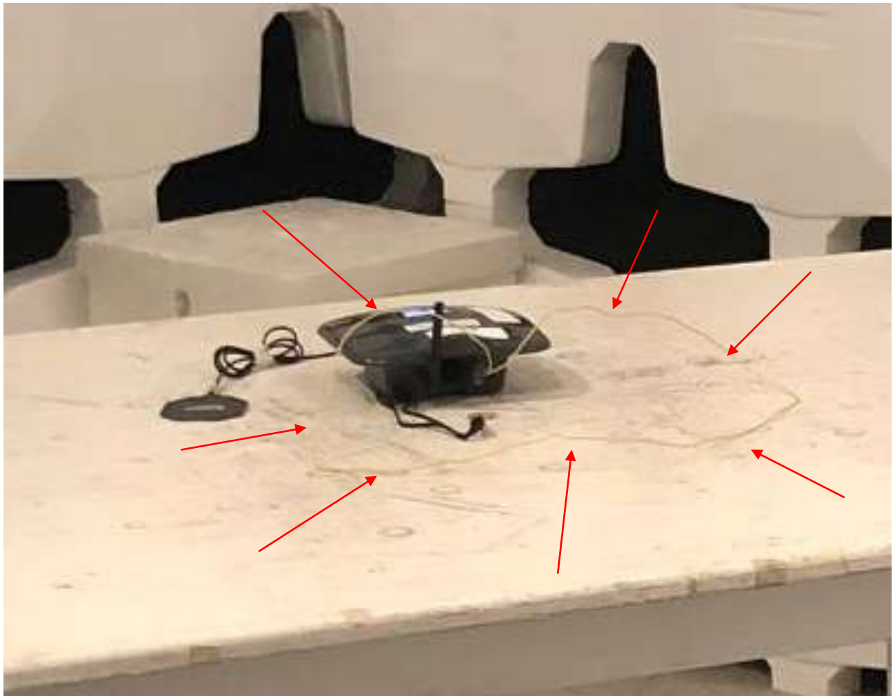
Figure 2. Close-Up of EUT on Table, showing Wire Loop Antenna
