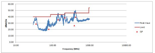
Figure 5. Radiated Emissions Graphical Data, 30 - 1000 MHz – Vertical
