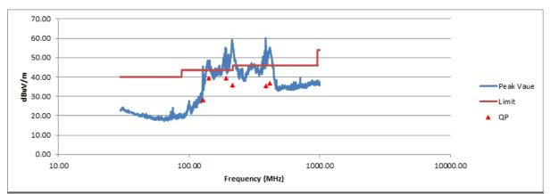
Figure 4. Radiated Emissions Graphical Data, 30 - 1000 MHz – Horizontal
