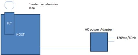
Figure 1. Block Diagram of Test Configuration (intentional)
