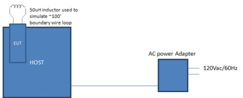
Figure 2. Block Diagram of Test Configuration (unintentional)
