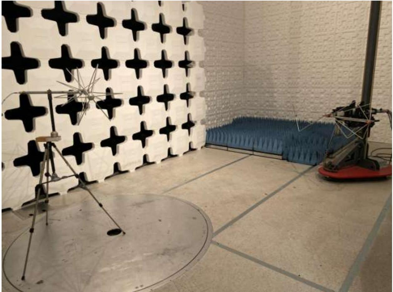
Figure 8. Substitution Testing (30-200 MHz)
