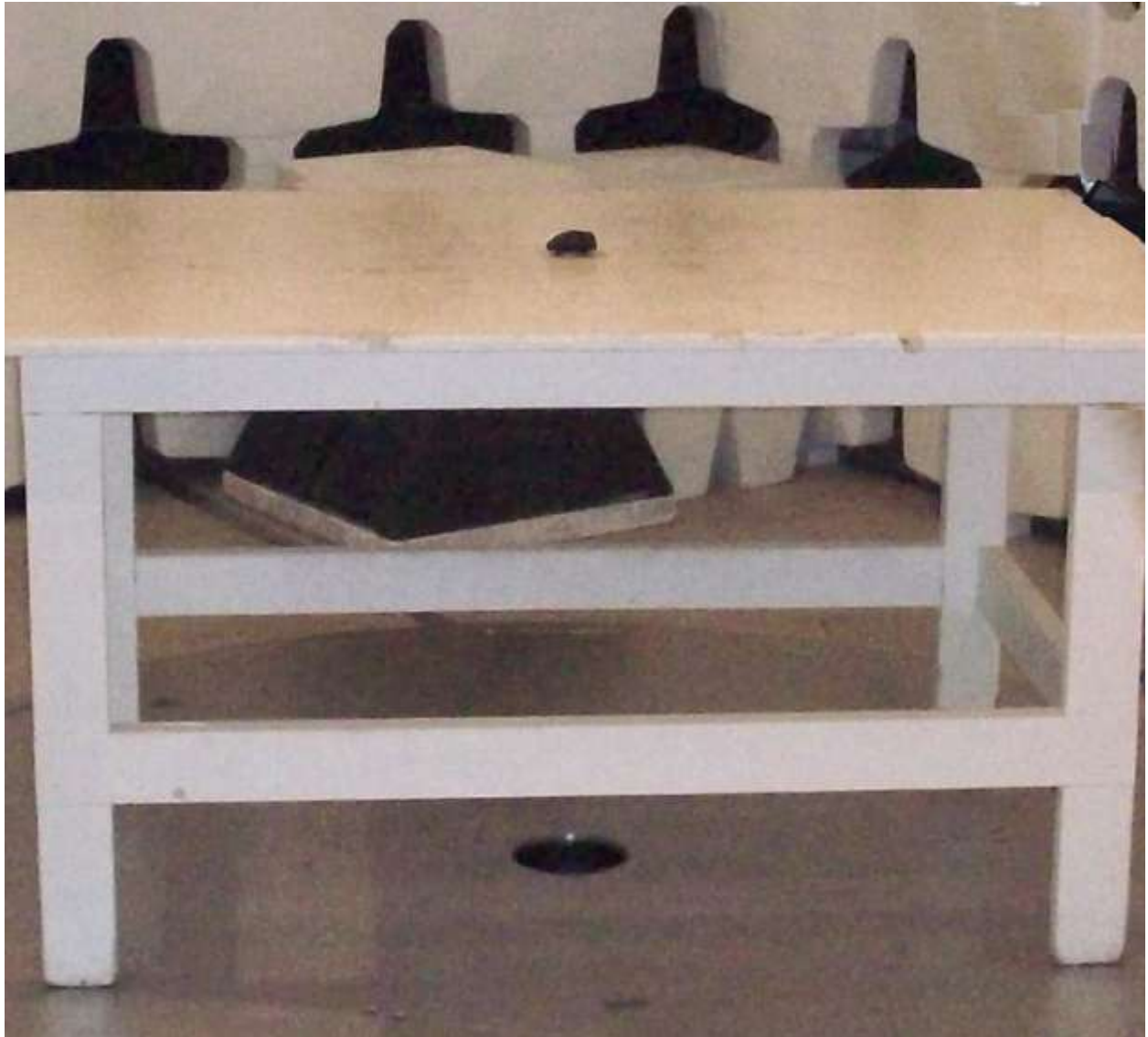
Figure 1. Radiated Emissions Test Setup
