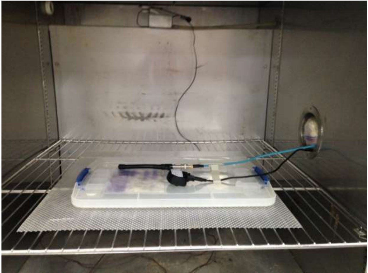
Figure 11. Frequency Stability Test setup
