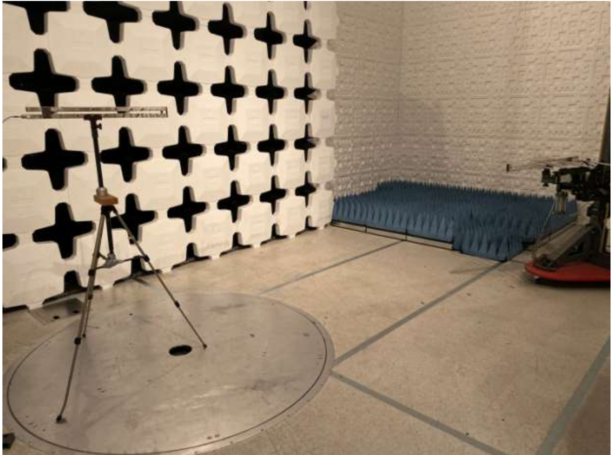
Figure 9. Substitution Testing (200-1000 MHz)
