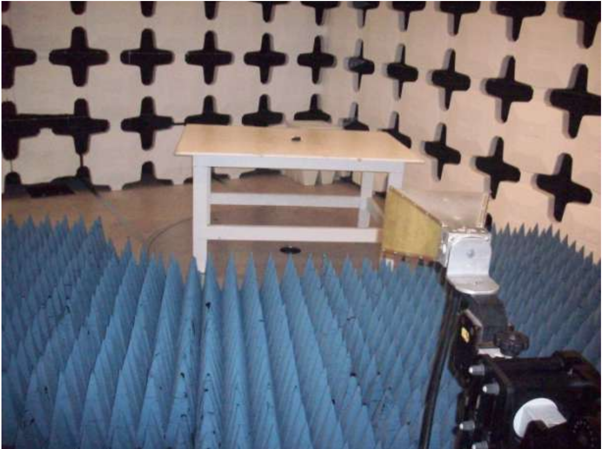
Figure 6. Radiated Emissions Test Configuration (Unintentional, above 1 GHz)
