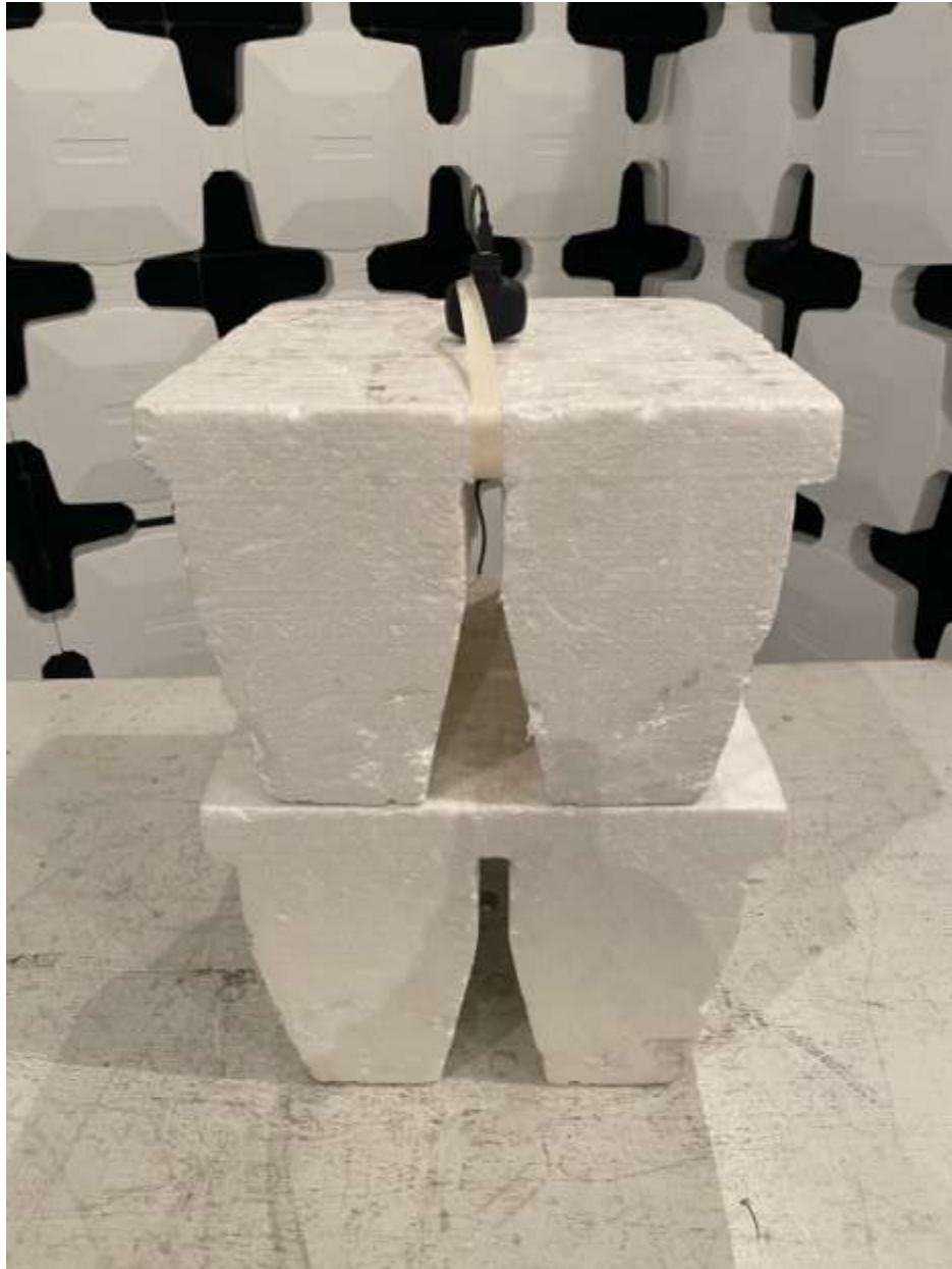
Figure 2. Intentional Radiated Emissions Test Setup (Above 1000 MHz)
