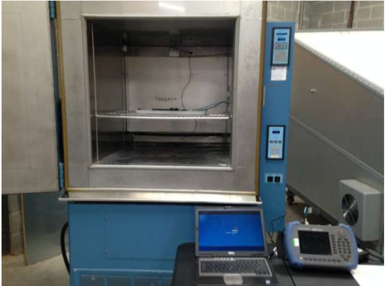
Figure 12. Frequency Stability Test Setup (Overall View)
