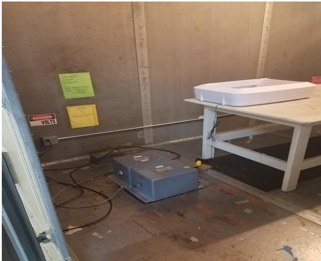
Figure 2. Conducted Emissions Test Setup
