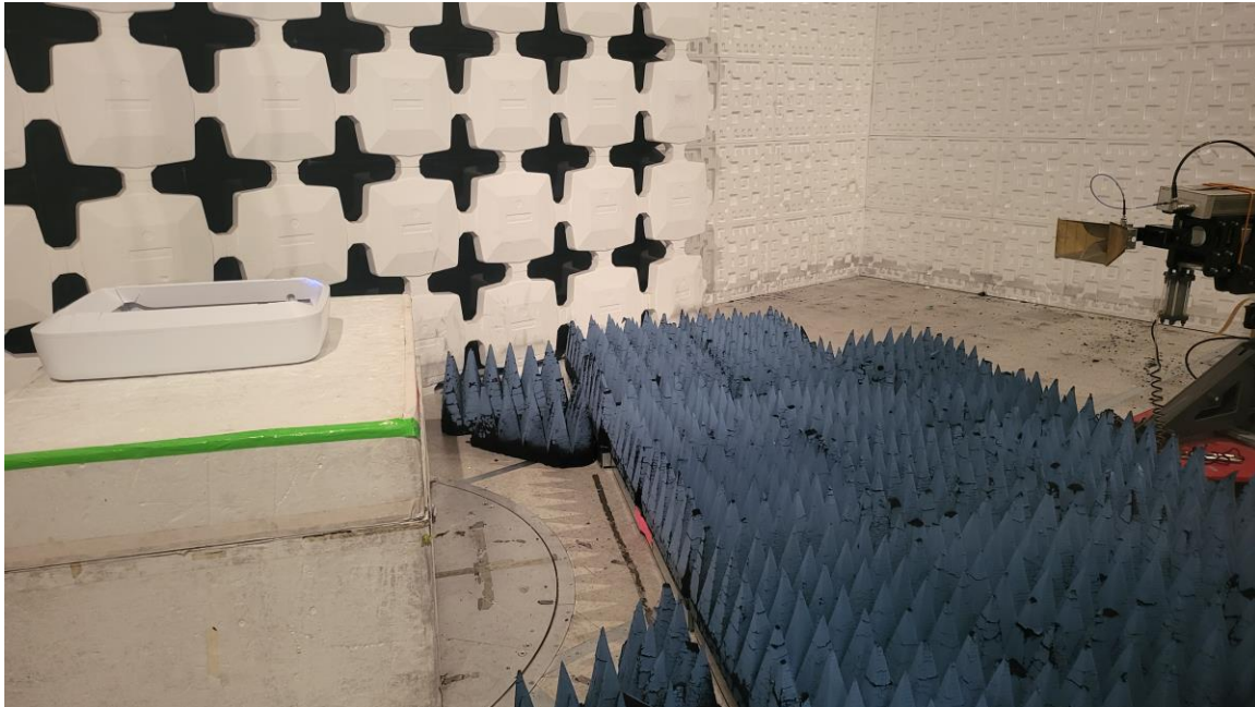
Figure 4. Radiated Emissions Test Setup, 1 MHz to 18 GHz
