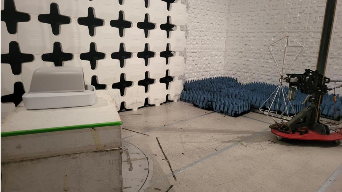
Figure 3. Radiated Emissions Test Setup, 30 MHz to 200 MHz
