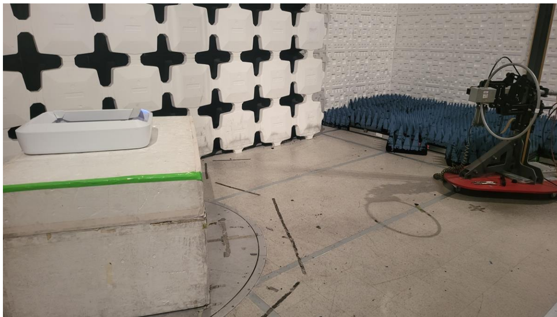
Figure 2. Radiated Emissions Test Setup, .15 MHz to 30 MHz
