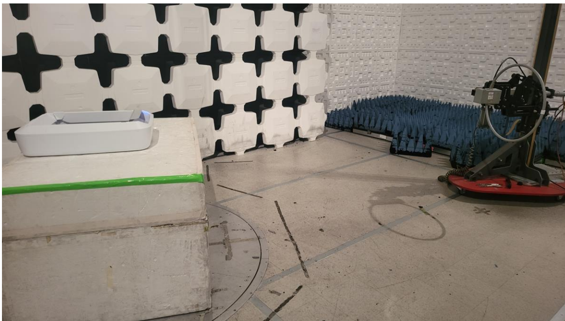
Figure 2. Radiated Emissions Test Setup, .15 MHz to 30 MHz
