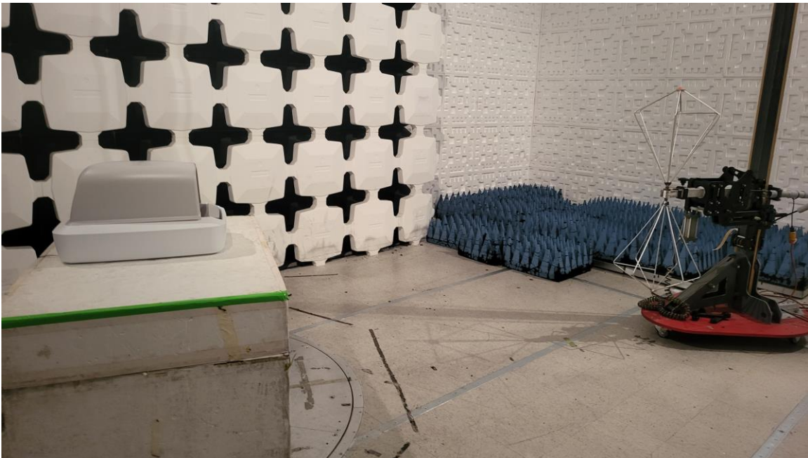
Figure 3. Radiated Emissions Test Setup, 30 MHz to 200 MHz
