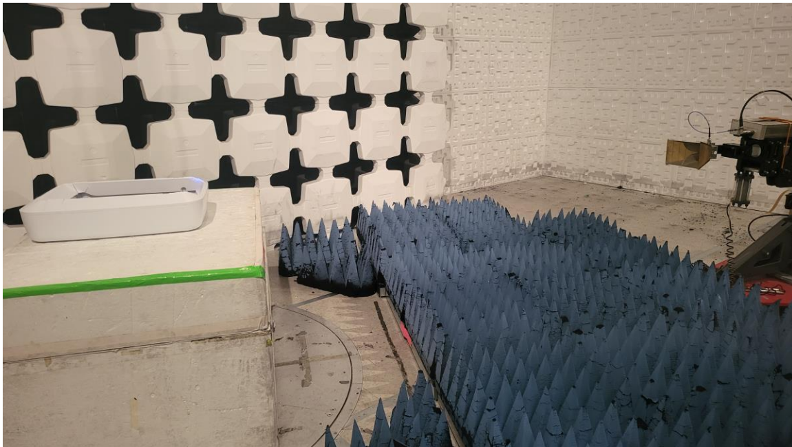
Figure 4. Radiated Emissions Test Setup, 1 MHz to 18 GHz
