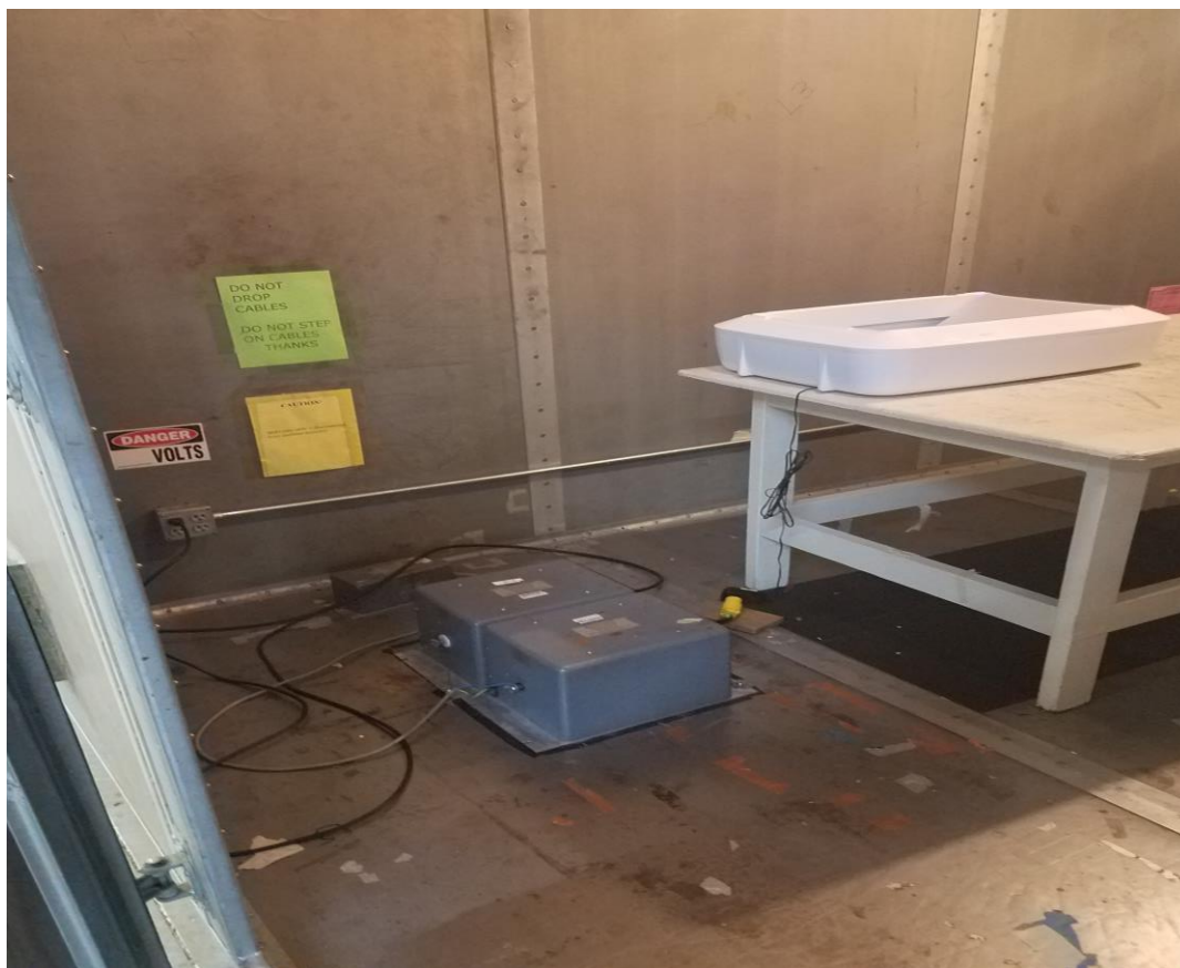
Figure 2. Conducted Emissions Test Setup
