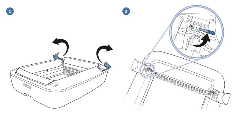
Unplug the litter box and remove the litter tray. Open the rake covers.
