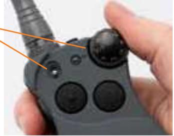
2. Press the mode button on the back of the Handheld with the tip of a pen. The Indicator Light will be solid green.
