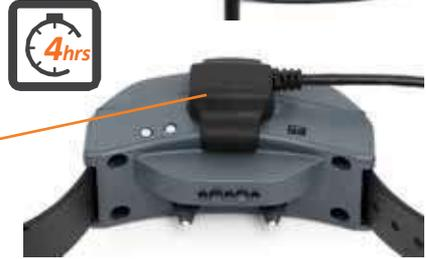
3. Connect each of the USB ends on the charging cables to the wall adapter and plug into a standard wall outlet. The Collar and Handheld Indicator Lights will be solid green while charging and flash green when fully charged.
