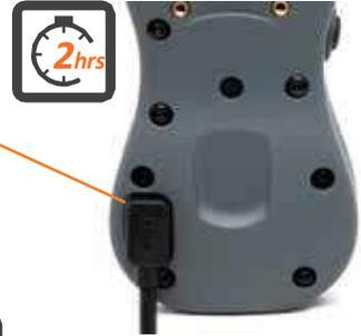
2. Snap the charging clip on the Collar by aligning the brass contacts on the clip to the connection points on the Collar and matching up the SportDOG® logos. The Collar takes 4 hours to charge.
